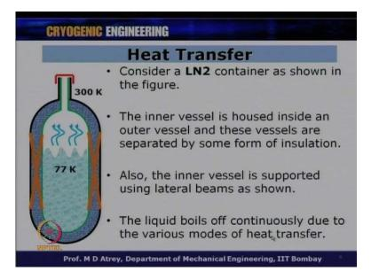
So, for example, we can see in a schematic, that we have got a  $\frac{1}{2}$  container outside temperature it is on 300 kelvin, and let us say liquid nitrogen here which is around at 77 kelvin. And this a open volume where the boil of would get stored. So, from 300 K to 77 K, we have got different ways in which the heat can transfer from outside to inside.
