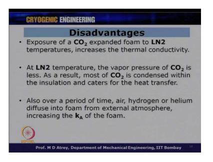
So, what are disadvantages: Exposure of a CO 2 for example, what is a gas being used, as I said CO 2. And once CO 2 get exposed to liquid nitrogen temperature, the CO 2 actually CO 2 will get condensed, it might it might get solidified; and this will increase the thermal conductivity. If I am talking about a temperatures level of LN2 in that case, thermal conductivity will increase.
