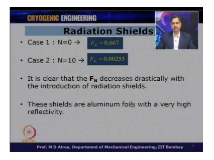
So, if I calculate all this things; what will get for the case one; when N is equal to 0 my F N will be equal to 0.667 and if I put N is equal to 10, my F N will be as small as 0.00255. So, its away from here, that if I put 10 shields of low emissivity and high reflectivity; my F N get drastically reduce my F e value now, will get drastically reduce from 0.667 to 0.
