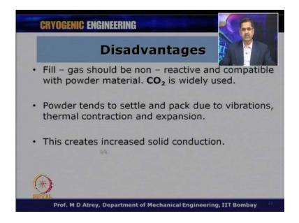
The disadvantages in this case the fill gas should be non reactive, and compatible with powder material CO 2 is again widely used. And this is true for earlier insulation also, that it should be a non reactive and compatible with powder material. The powder tends these are one of the disadvantages; the powder tends to settle and pack due to vibrations, thermal contraction and expansion.
