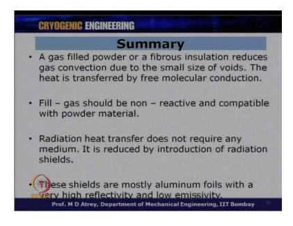
A gas filled powder or a fibrous insulation reduces gas convection due to the small sizes of voids. So, you have got a very small particulate matter particles sitting over there, in which there to be gas; and this will effectively reduce the apparent thermal conductivity from 30 to 55 mille watt for expanded foam to around 20 to 35 for gas fill powder case. The heat transfer is reduce by free molecular is transfer happing, because of free molecular conduction in this case.
