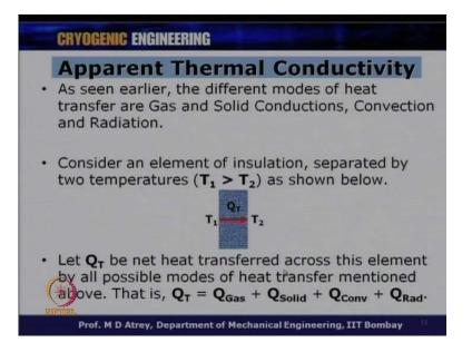
So, as seen earlier the different modes of heat transfer are gas and solid conduction, convection, and radiation; consider an element of insulation separated by 2 temperatures. Lets say T 1 and T 2, and which case T 1 is more than T 2. So, here is what we can see that one surface is at T 1, the other surface are T 2. And Q 1 is the conduction, Q 1 is basically the heat that is being transferred from this surface to other surface alright.
