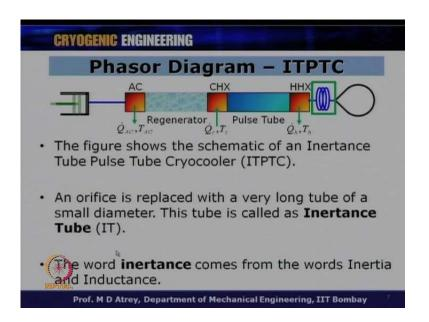
So, this is my inertance tube pulse tube cryocooler. We got a (()) after cooler, regenerator, cold end heat exchanger, pulse tube hot end heat exchanger, and this hot end heat exchanger in a OPTC will be connected through an or (()) to a reservoir. Now, I am getting read of orifice, and I will have a inertance tube which is a small diameter kind of a capillary tube running into length, of let us say 1 meter to 2 meter depending on the diameter, and it get in connected to a reservoir.
