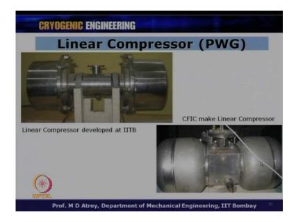
The compressor I use or a pressure we have generator, which I use is a linear compressor. The linear compressor work on the principle of linear motor; and this is the
