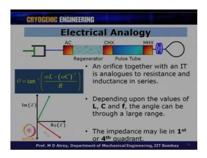
And for a inertance tube now, I want to prove that an orifice together with the inertance tube now is analogous to resistance and inductance. It has got small opening. So, we got a inductance, capacitance alright; so, we got a RLC circuit over here, now and in this case my tan theta will be omega L minus omega C inverse divided by R; depending upon the value of LC and f the angle can be changing through a large value now.
