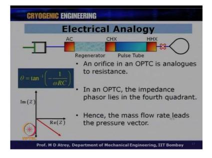
Now, let us have a Orifice; let us see this electrical analogy to OPTC and ITPTC. So, an Orifice in an OPTC analogous to resistance; so, we got a theta is equal to tan inverse of minus omega RC, this is what we had seen; and here now we know that the current the impedance lies in the 4 th quadrant, we had seen these and in this case now we know that mass flow rate leads the pressure vector.
