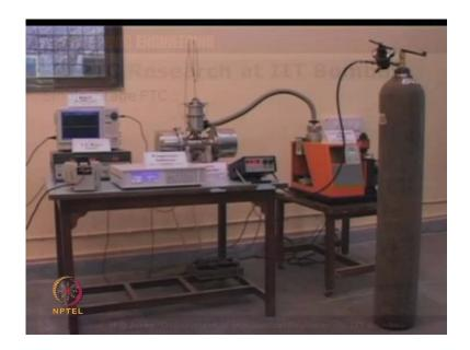
So, here I got a small video of the pulse tube refrigerator that has been developed in our laboratory. Our past research student (()) narayan (()) also has worked towards making this pulse tube refrigerator at IIT Bombay. So, this my pulse tube refrigerator, and this is the linear compressor.
