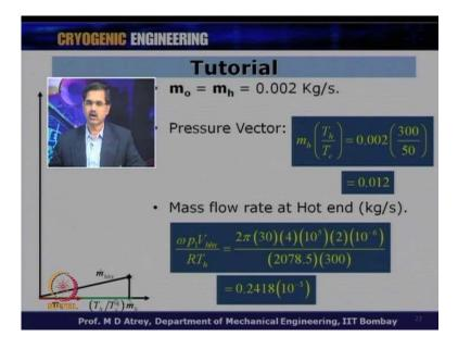
So, begin with I know m dot o is equal to m dot h for OPTC which is given as 2 gram per second, which is 0. 002 K g per second. Then, we know the pressure vector is going to
