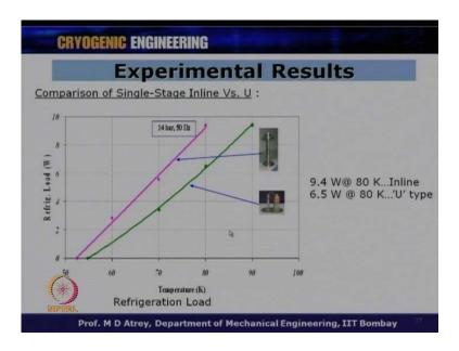
Now, I (()) want to see the cooling effect also. So, what I do normally I will put a electrical heater at the other end or the cold end; and I will go on increasing the wattage which will actually acting as the dummy load in a system, and this will give you basically what is the wattage or a cooling load delivered from a system.
