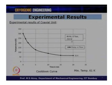
And now, I have got a coaxial unit again here; I reach around 61 kelvin temperature, but you can see how fast I have reached here. Basically, in almost 20 minutes, so I have got a operation at 46 hertz, but I got 17 bar higher pressure little bit as complete to earlier case, and power input of 250 watts.
