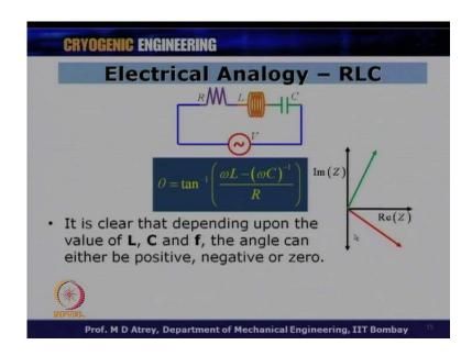
So, theta is going to be tan inverse of omega L minus omega C inverse divided by R; and depending on the value of this, I can have a theta from positive to negative; that means, I can have Z vector in the first quadrant, and also in the 4 th quadrant; I have got all the possibilities depending on the value of the inductance, the omega and the capacitors.
