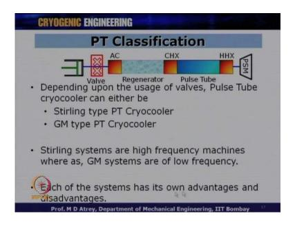
Now, let us see this classification in little more detail. So, as you know that depending on the usage of valve the pulse tube Cryocooler can either be Stirling type pulse tube cooler or a GM type pulse tube cooler. The moment as a GM type pulse tube cooler I got a wall over here Stirling systems are high frequency machines whereas, GM systems are low frequency machine I hope this is now, entirely clear to all of you each of the system as know earlier is at got own advantages and disadvantages.
