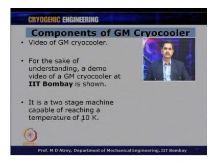
It is a two stage machine which is capable of reaching a temperature of around 10 Kelvin, the lowest temperature possible is around 10 Kelvin, but normally it is referred to as 10 Kelvin cryocooler, 10 Kelvin machine.
