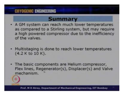
A GM system can reach much lower temperatures as compared to Stirling system, but may require a high powered compressor due to the inefficiency of the valves. Multistaging is done to reach lower and lower temperatures you can get less than 4.2 Kelvin or a 10 Kelvin system whatever you want. The basic components of a GM cryocooler are Helium compressor, Flex lines regenerators and displacer valve mechanism etcetera.
