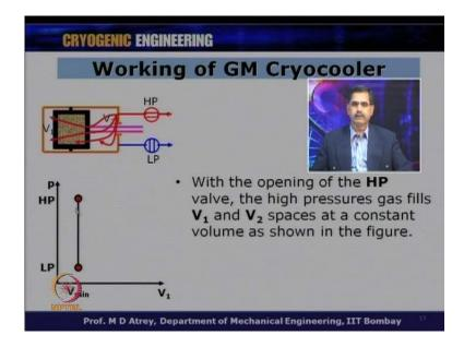
So, now you can see that I have made the high pressure gas open, I have made the HP valve open with the opening of this HP valve, the high pressure gas fills V 1 and V 2. So,
