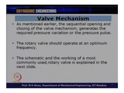
As mentioned earlier, the sequential opening and closing of the valve mechanism, generates the required pressure variation or the pressure pulse. The rotary valve should operate at an optimum frequency. We have seen that the GM cooler functions at 1 to 2 hertz or 1 to 3 hertz. Let us say this optimum frequency's very important at what
