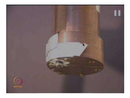
So, here in the second stage whatever you want to cool will be conductively coupled in the second stage of the GM cryocooler.
