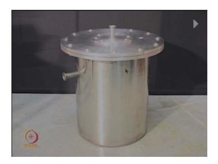
Now, if I want to test the performance of the GM cryocooler, we have made this vacuum jacket and in this vacuum jacket this two stage GM cryocooler will be put in. So, this flange can be taken off and the flange with GM cryocooler can be put in this case. So, this is basically about a vacuum jacket to test the performance of GM cryocooler.
