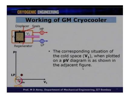
I would like to show now, what is how the pressure v, pressure versus volume diagram changes with this motion of displacer and we are talking about this volume V 1. So, at present we have got a v minimum this and the gas let us say at low pressure is there at V 1. So, corresponding situation of the cold space V 1 when plotted on a pV diagram is as shown in the adjacent figure, as shown over here.
