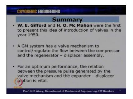
Summarizing Gifford and McMahon were the first to present the idea of introduction of valves in 1950. A GM system has a wall mechanism to control/regulate the flow between the compressor and the regenerator-displacer assembly. For optimum performance the
