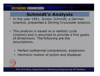
So, in the year 1861, Gustav Schmidt, a German scientist presented a Stirling Cryocooler analysis. This analysis is based on realistic cycle that is from motion point of view as we saw that discontinuous motion is not possible and Schmidt considered a continuous motion or a sinusoidal motion, which is the more realistic kind of a motion. And we assumed that this motion to provide a first guess of dimension; the following are different assumptions.
