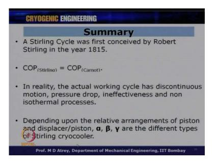
So, in summary, I were to write the summary of this lecture; a Stirling cycle was first conceived by Robert Stirling in the year 1815; we know that COP Stirling is equal to COP carnot; in reality, the actual working cycle has discontinuous motion, pressure drop, ineffectiveness and non isothermal process; depending on the relative arrangement of piston and displacer/piston, alpha, beta, gamma are different types of Stirling Cryocoolers.
