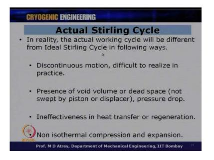
Actual Stirling cycle in reality the actual working cycle may be different from ideal Stirling cycle in following ways. So now, what we are doing we are going away from ideal Stirling cycle; and we are talking about in what ways, the actual Stirling cycle could be different than ideal Stirling cycle. What are different possibilities; the first possibility we just pointed out is a discontinuous motion, it is difficult to realize in practice.
