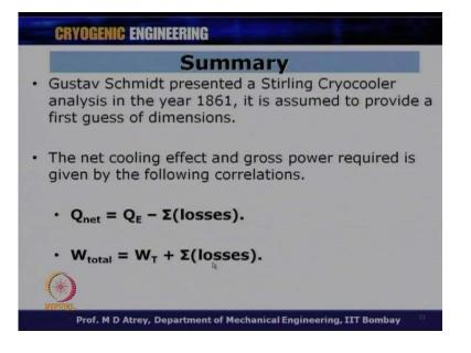
Schmidt's presented a Stirling cycle analysis in the year 1861, it is assumed to provide a first guess of dimensions. The net cooling effect and gross power input is given by following correlations; Q net is equal to Q E minus sigma losses; W total is equal to W T plus sigma losses. A self assessment is given based on this lectures, kindly assess yourself for this lectures.
