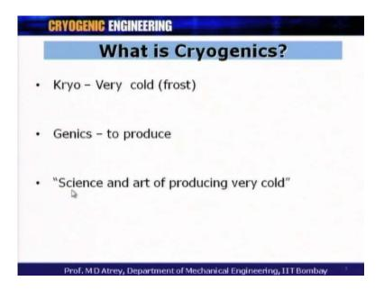
What is Cryogenics? Kryo is very cold, as cold as ice although cryogenic means very low temperature, but the name is coming from as cold as ice. Then Genics is to produce. So, basically cryogenics is nothing but science and art of producing very cold, that is what find earlier and still today the definition carries.
