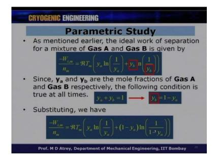
So, as mentioned earlier, the ideal work of separation for a Gas mixture Gas A and Gas B is given by this formulae which we know about. Since, Y a and Y b are the mole fraction of Gas A and Gas B respectively, the following condition is always true at all the times. Y a plus Y b is equal to 1 and therefore, Y b can be always be 1 minus Y as if I put this two values and this is possible when I am talking about two Gas mixtures Gas A and Gas
