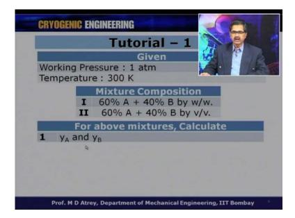
So, working pressure is one atmosphere, temperature is 300 Kelvin, the mixture compositions in the case one, 60 percent A and 40 percent B by weight, weight of A and B per weight of mixture or 60 percent A plus 40 percent B by volumetric basis. For above mixtures, calculate Y a and Y b, what are Y a and Y b? That the mole fractions of A and B that you got the problem statement is.
