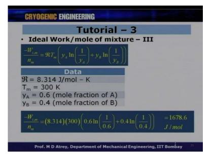
The data is plotted graphically, in further slides. So, let us first calculate ideal work requirement per mole of mixture for case three. So, this our formulae which is very well known. Now, the data is given and for case three, Y a is 0.6 that is 60 percent of a and 40 percent of b 0.6 and 5.4. So, calculate W i m by n m, put this 0.6 1 by 0.6 0.4 log 1 by 0.4 the answer is 1678.6 joule per mole of mixture. So, work of separation is this quantity for 60 40 cases.
