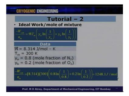
All right, so, ideal work per mole of mixture which is W i m upon n m and this is standard formulae. So, basically now, put the values. So, we know r is universal Gas constant 8.314 t m is equal to 300 Kelvin Y a is 0.8, Y b is 0.2. Putting these value W i m upon n m is equal to this formulae 0.8 log 1 by 0.8, 0.2l go 1by .2 into R T m and this is giving you1248.1 joule per mole.
