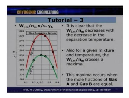
Meaning which directly that the work of separation requirement is less for 200 Kelvin than at 300 Kelvin and this is what our first conclusion should be. It is clear that work of separation per mole of mixture decreases with the decrease in separation temperature and this is clear from the formula itself. Now, what is to be understood is also for a given mixture and temperature the W i m upon n m crosses a maxima, which is what you can see, the maximum here, the maximum here.
