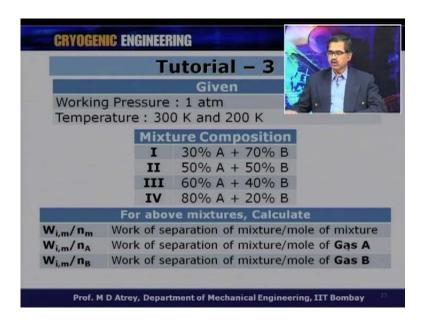
The mixture compositions are case one, case two, case three, case four and for above mixtures calculate W i m by n m which is work of separation of mixture per mole of mixture W i m by N A work of separation of mixture per mole of Gas A W i m by N B.
