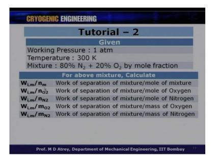
So, what are the data given which is the working pressure 1 atmosphere, temperature 300 Kelvin, mixture 80 percent, nitrogen and 20 percent, oxygen by a mole fraction. So, Y a is 0.8 Y b is 0.2. Now, the nomenclature that we are going to follow from this lecture onwards is to understand this and these are the terms which normally be used. So, what
