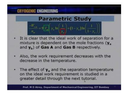
So, I can understand from this figure that it is clear that the ideal work of separation for a mixture is depends on mole fraction that is Y a and Y b on Gas A and Gas B respectively, also the work requirement decreases with the decrease in temperature you can see the t m value over here. So, depending on what is my quantity of Y a and Y b, the ideal work of separation will be vary. Also depending on the temperature is what the temperature of separation is the W i m by n m value will vary.
