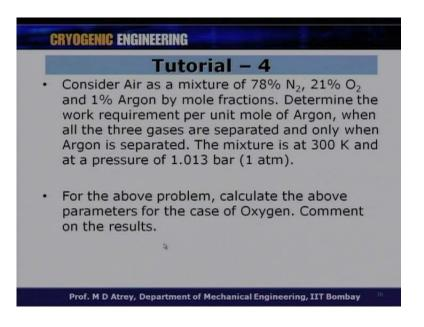
Determine the work requirement per unit mole of argon, when all the three gases are separated and only when argon is separated. That means, first case is what is work of separation per unit mole of argon and second thing is what is the work of separation when only argon is separated from this mixture of three gases. The mixture is at 300 Kelvin and at a pressure of 1.013 bar.
