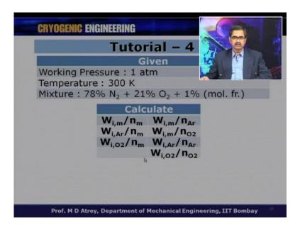
So, what are the parameters given? Working pressure is given, temperature is given, and the mixture composition on molar basis is also given. So, what are the molar basis? 78 percent nitrogen 21 percent oxygen 1 percent argon.
