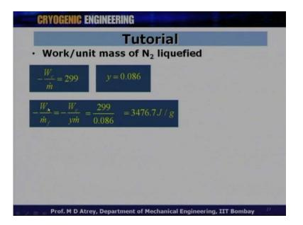
And work done per unit mass of gas liquefied is W c y m dot is equal to 299, y is equal to 0.086 and W c by m dot f is 299 upon 0.086 which is 3476.7 joule per gram all right. So, what you get from here is? The work done on compression per unit mass of gas which is liquefied.
