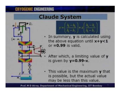
In summary, how do I calculate y. Y is calculated using the above equation until x plus y is less than 1 or 0.99. So, this expression is valid, when x plus y is equal to 0.99. After which, a limiting value of y can be calculated by y is equal to 0.99 minus x and this is what a general principle, we are going to follow to calculate the yield choosing Claude cycle I would this clear to you.
