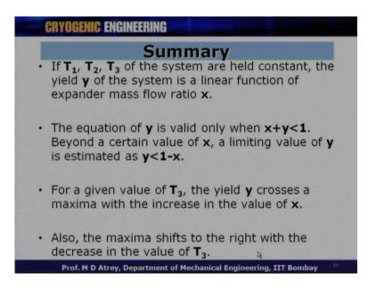
If T 1, T 2 and T 3 of the system are held constant, the yield y of the system is a linear function of the expander mass flow ratio x. Again, this is clear from the yield expression for y.
