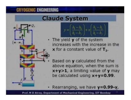
The yield y of the system increases with the increase in the value of a x for a constant value of T 3, that is what we have seen that. If we start increase the value of x from let say point 1 at a particular value of T 3, it will start increasing with a value of x in a linear fashion.
