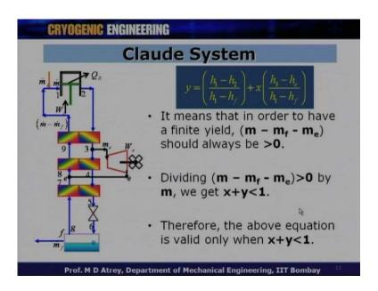
So, it means that in order to have a finite yield; that means, in order to have a finite value of y at this point your m minus m f minus m e which is nothing, but the return stream at point g has to be always more than 0; that means, it should be some finite value so, that the heat exchangers function.
