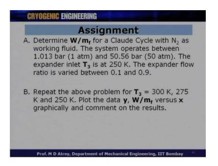
With this background and with this tutorial an assignment is given to you on the similar line (()) Nitrogen as a working fluid, but we have changed the pressure to 50 atmosphere and again T 3 has to be 250 Kelvin, expander flow rate to be varied from 0.1 to 0.9.
