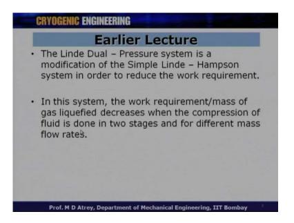
Then we went for a Linde Dual - Pressure system wherein, we used two compressors. The Linde Dual - Pressure system is a modification of the simple Linde - Hampson system in order to reduce the work requirement. In this system, the work requirement per mass of gas liquefied decreases when the compression of the fluid is done in two stages and for different mass flow rates. I think this is very straight forward and this is what we did during the last lecture?
