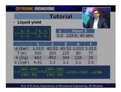
So, let us start doing simple calculations and calculate the liquid yield by the formula y is equal to h 1 minus h 2 upon h 1 minus h f plus x time h 3 minus h e upon h 1 minus h f. Where, x is equal to 0.2 in this case, T 3 is equal to 225 Kelvin and 40 atmosphere pressure.
