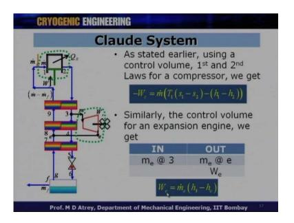
As we have stated earlier, using the control volume first and second law for compressor. This is very standard equation, which we have use almost in the of the cycles that work done on the compression is equal to m dot into T 1 into delta s across 1 and 2 minus delta h across 1 and 2, the very standard, equation which has been used.
