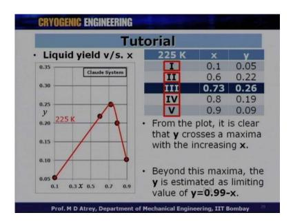
So, if I plot this thing that is y versus x what we have just calculated and I just take 4 representative values or 5 representative values over here and if we calculate case number 1, 2, 3, 4 and 5 and what if I join what you say is? This is the x, when the x is varied from 0.1 to 0.9 y goes to a maxima and the maximum value happens to be around 0.25 or 0.26 for T 3 is equal to 225 Kelvin temperature.
