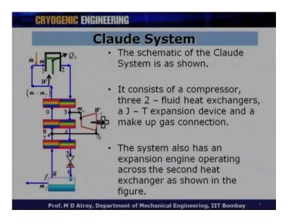
So, this is a schematic of a Claude cycle and what you can see from here. It has got a compressor over here and it has the... What an expander over here? And we got a heat exchangers 1, 2 and 3 and there is the J - T wall at the end whether liquid is yielded in a container at this point here.
