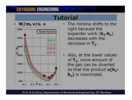
The minima shift to the right, because expander work h 3 minus h e decreases with the decrease in the value of T 3. Also, at the lower values of T 3, more amount of the gas can be diverted so, that the product x into h 3 minus h e is maximized. This is what we talked about earlier for the y versus x case? And this is what has to be well understood, that y it goes to a minimum and y it shift to right in this particular case.
