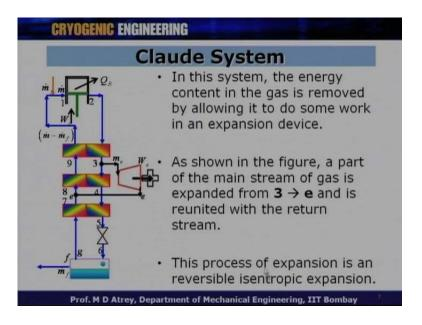
So, in this system, the energy content in the gas is removed by allowing it to do some work in an expansion engine. So, what you get at the end of the expansion over here is W e, which is the expansion work that is the work done by the expansion engine. So, here on the compressor, we are doing the work while at this point here during expansion we get W e as the work done by the system.
