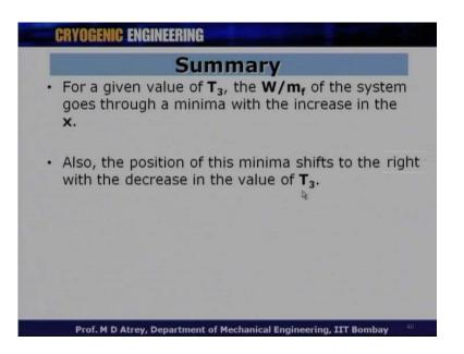
For a given value of T 3, the W by m f of the system goes through a minima with the increase in the value of x and this is again the optimum value of x, we would like to attain or use for design purpose for cycle optimization. Also, the position of this minima shifts to the right with the decrease in the value of T 3.
