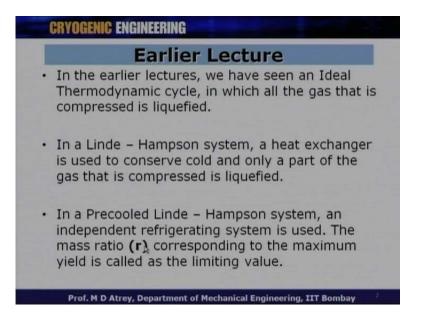
In the earlier lectures on gas liquefaction, we have talked about various cycles and I will just go in brief about those cycles. We have seen an ideal thermodynamic cycle, in which all the gas that is getting compressed is getting liquefied. In the ideal cycle, whatever gas gets compressed, it gets liquefied 100 percent.
