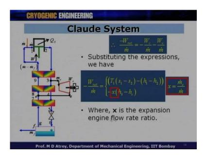
So, if I put them together, I will get dividing by m dot to the expression. I get W net upon m dot; that means, net work done per unit mass of gas which is compressed is equal to T 1 into s 1 minus h 2 minus h 1 minus h 2 minus x into h 3 minus h. Where, x is equal to m dot e upon m dot again, x is the expansion engine flow rate.
