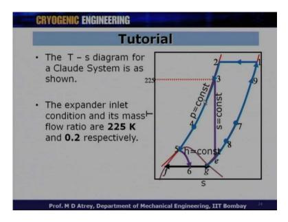
Now, one can see the corresponding T - s diagram here. 1, 2 is a compression, 2 to 3 is a cooling, 3 to e is where you get the point e that is what I just said, that we draw a vertical from high pressure line at point 3 to the low pressure line which intersect this point at e and correspondent to this what you get is 80 Kelvin in this step. In this particular case, temperature at point 3 is 225 Kelvin.
