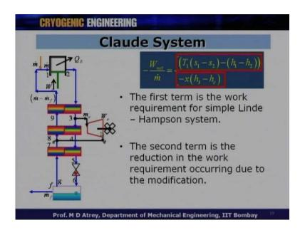
So, what do we understand from this? The first term is the work requirement for simple Linde - Hampson cycle, where the only compressor comes into picture. While, the second work is the work done by the system and it is coming only, because the
