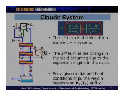
So, the first term is the yield of a simple Linde - Hampson cycle, which we have seen that it depends only on the point 1 and 2, the compression process 1 and 2. The second term which is an addition to the simple Linde - Hampson cycle is basically coming, because of the expansion engine over here. So, second term is the change in the yield occurring due to the expansion engine in cycle.
