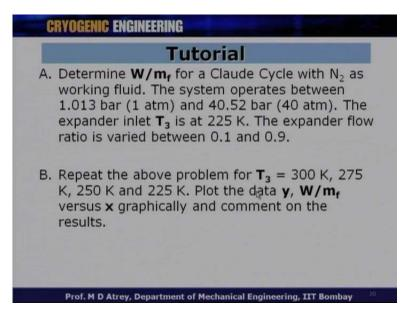
So, from that point of view this tutorial has been framed. The part a is determine W by m f that is work of compression per mass of gas liquefied for a Claude cycle with Nitrogen as a working fluid. So, one can have air Oxygen, Nitrogen etcetera with Nitrogen are the working fluid in this case. The system operates between 1 atmosphere and 40 atmosphere or 1.013 bar and 40.52 bar. The expander inlet T 3 value is 225 Kelvin that means it is below ambient.
