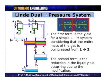
That means, that y is equal to this expression and what you have is the first term is the yield for a simple Linde - Hampson system considering that entire mass of the gas is compressed from 1 to 3. So, if you look at this first term it is nothing, but this that is a simple Linde - Hampson system. Where, the gas is compressed within 1 compressor from point 1 to point 3 and the yield in that case would have been this.
