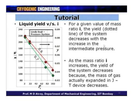
So, for a given value of mass flow ratio i, the yield of a system decreases with the increase in intermediate pressure. Why does it happen? Now, if you recollect the expression for y, we have got the first term and the second term. What you understand second term, has a negative value which has numerator as h 1 minus h 2 as you understand that as the value of P 2 of the P i increases, this second bracket starts increasing and therefore, the value of y decreases all right.
