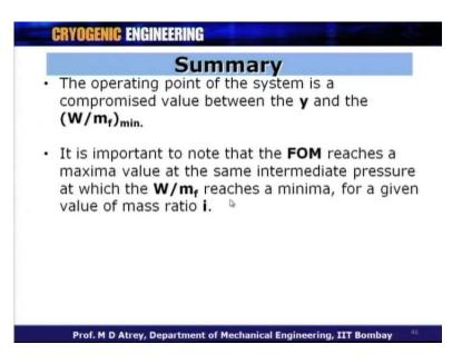
The operating part of the system is a compromised value between y and W upon m dot f, as you know as you go on increasing the intermediate pressure the value of y decreases. But the value of W by m dot f will fall through minima. So, one has to taken optimum value between 2 between in this 2. In fact, why should design to gate W by m dot f minimum corresponding to that your desired y value should match.
