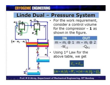
For the work requirement now, what we have done till now is a finding an expression of y. But what is most important is? What is my W c 1 and W c 2? Which is the work input to the compressor number 1 and the work input to the compressor number 2 and this is what will basically bring about the advantages, we get in a Linde - Dual pressure system.
