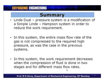
In summary on this particular lecture, the Linde Dual - Perssure System is a modification of a simple Linde - Hampson system in order to reduce the work requirement all right.
