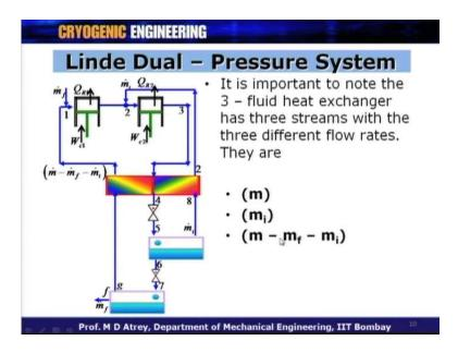
It is important to note that 3-fluid heat exchanger has three streams with the three different flow rates. They are as I just talked about m dot which is coming from here m dot I which is going back and m minus m f minus m I which is going through this point.
