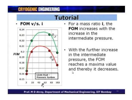
So, for mass ratio of i the Figure of Merit increases with the increase in the intermediate pressure. With the further increases in the intermediate pressure, the Figure of Merit reaches a maxima value and thereby it decreases.
