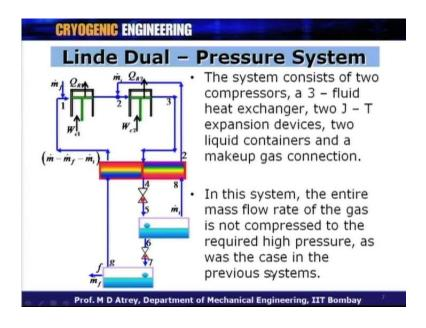
So, here is a slide which shows you how a Linde Dual - Perssure System works. So, as I said dual means 2 and we have got 2 compressors. This is what you can see from this particular schematic? There are 2 compressors and 2 expanders. So, we have got 2 compression processes and we have got 2 expansions over here at the same time, we have got 2 containers also.
