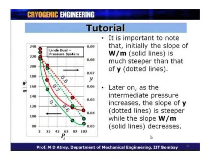
It is important to note that, initially the slope of W by m dot is much steeper than that of y. Later on, as the intermediate pressure increases, the slope of y is steeper while the slope W by m dot decreases in this case.
