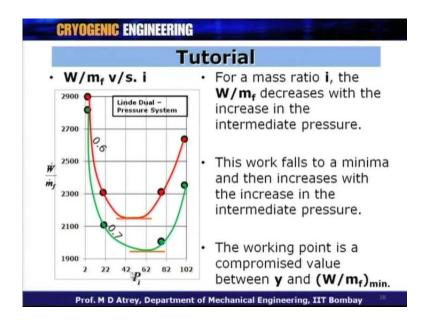
For a mass ratio of i , W by m dot f decrease with the increase in the intermediate pressure. It decreases first goes through minima and again starts increasing. The work falls to minima and then increases with the increase in the intermediate pressure and you can find that for this case 0.6, one should operate at a pressure somewhere around 50 bar, 50 atmosphere while somewhere on 62 is a corresponding optimum pressure for i is equal to 0.7.
