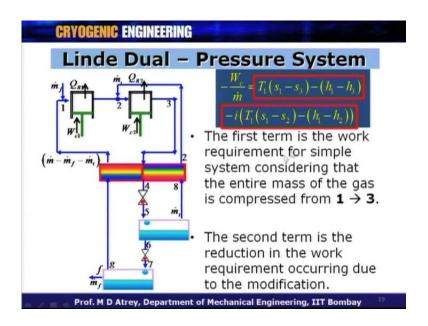
So, same thing is written in the first term, is the work requirement for simple system considering that the entire mass of the gas is compressed from 1 to 3.
