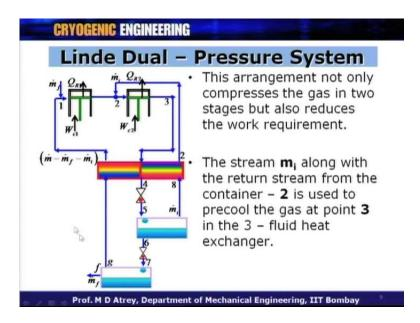
This arrangement not only compresses the gas in two stages, but also reduces the work requirement and this is why we are doing all this thing? Basically, we want to reduce the work done per unit mass of gas which is compressed. The stream m dot i along with the return stream from the container number 2 here, is used to precool the gas at point 3 in the 3-fluid heat exchangers.
