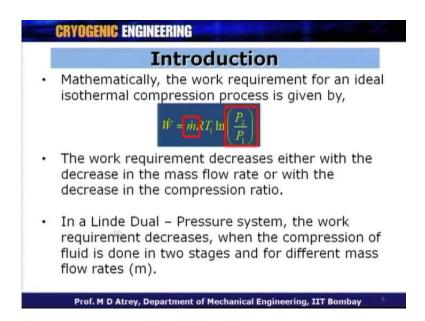
Mathematically, the work requirement for an ideal isothermal compression is process given by W dot is equal to m dot r T 1 lock P 2 by P 1. This is the work of compression for an isothermal process. What does this mean? The work requirement decreases either with the decrease in mass flow rate or with the decrease in compression ratio. In this equation, you can see there are 3 parameters m dot T 1 and P 2 by P 1.
