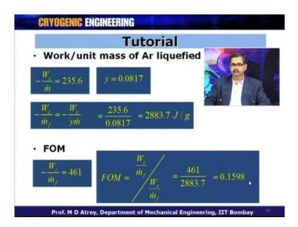
Now, I want to calculate work done per unit mass of Argon liquefied for which what I want to know is? W c upon m dot and I want to know what is the value of y? Which is 0.0817 which is what we have just calculated? What we know is? W c upon m dot f is equal to W c upon m dot upon y all right. So, what we have is both the values? This upon this will give you W c upon m dot f.
