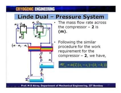
The mass flow rate across the second compressor is m dot. Following the similar procedure for the work requirement for the compressor 2, what we get is? minus W c is equal to m dot into T 1 into s 2 minus s 3 minus h 2 minus h 3, because the process W c 2 compression processes happening across point 2 and point 3 and we are taking the entropies and enthalpies related to those point. So, this will form the work of compression for the second compressor.
