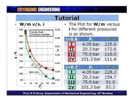
Now, let us plot the second parameter which is W by m dot versus I all right. So, the plot between W by m versus i for this value is over here. So, we got a various values and you can see that as you gone increasing the value of intermediate pressure, the W by m dot decreases. What is important node is? The slop of this is much higher initially, while it is less and less as you go for higher value of intermediate pressure.
