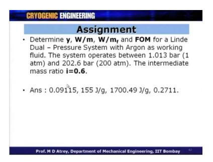
I got a assignment for you and assignment solving only this will make you perfect. So, what I want to you understand solve the problem again, for Argon for different pressures of 1 bar and 200 bar. Now, intermediate mass ratio is taken as 0.6 and we have go in the answers also for this case for y W by m dot W by m dot f and Figure of Merit. So, please do this in this size and check your answers, check your calculations to get these answers.
