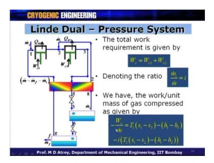
Now, the total work requirement is given by W c is equal to W c 1 plus W c 2. So, the total work is now going to be determined by what is the value of W c 1? And what is the value of W c 2?W c 1 depends on what is the amount of gas which is getting compressed in the compressor number 1 and what is the pressure ratio across point 1 and 2 all right P 2 by P 1.
