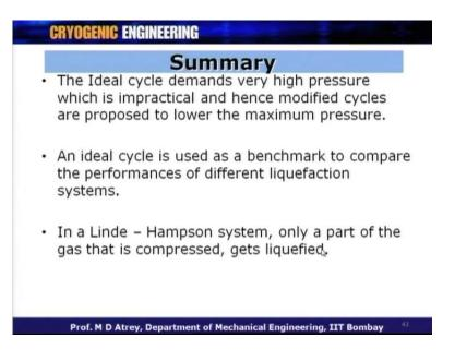
A heat exchanger is used in a Linde - Hampson system to conserve cold in the system. This process is an isobaric process, and is assumed to be 100% effective.
