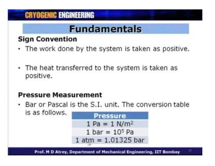
With these parameters, now let us see some fundamentals, which would help us to finalize the liquefaction cycle. The sign convention that I just talked about is that, the work done by the system is taken as positive. Similarly, the work done on the system will be taken as negative. The heat transferred to the system is taken as positive, and the heat leaving the system will be taken as negative.
