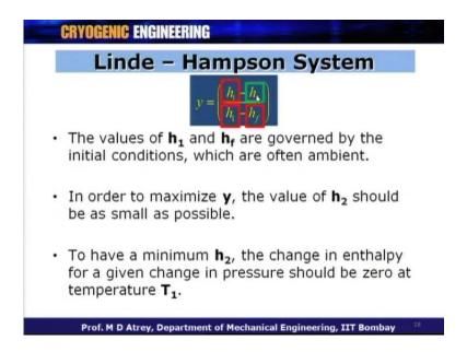
Here we can see that the values - h 1 and h f, are governed by the initial conditions, which are often ambient condition. So, h 1 is corresponding to 1 bar, and 300 k; corresponding to 1 bar, h f dot will be at 77 Kelvin, which is the boiling point of liquid nitrogen, at 1 bar pressure.
