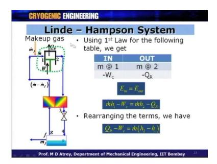
Using the first law, for the following tables, whatever is coming in, is equal to whatever is going out; as E in is equal to E out. We can find out that, therefore, m dot h 1 minus w c is equal to m dot h 2 minus q r. If we rearrange these terms, what we get is q r minus w c, is equal to m dot into h 2 minus h 1.
