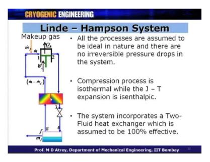
We have just seen that all the processes are assumed to be ideal in nature, and there are no irreversible pressure drops in the system. This is the assumption which will be used for analyzing this system.
