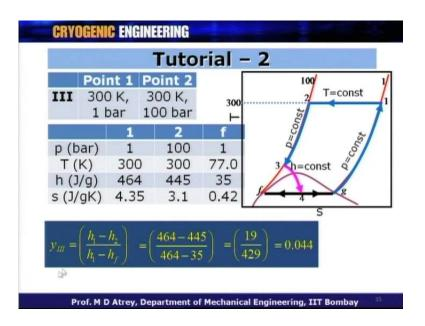
Let us go to case number 3, which is happening at 300K. The process of compression is happening at 300K only; but the pressure at the end of compression is now 100 bar, and not 50 bar anymore. Correspondingly, now I have got point 1 at 1 bar, and point 2 is at 100 bar, and 300 Kelvin.
