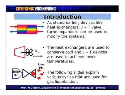
In the first lecture, I had talked about heat exchangers like, joule Thomson valve, and turbo expanders, all these systems could be used to modify the system, and now that we talked about changing the ideal thermodynamic cycle to get a relatively practical cycle, we will have to use all these components as a two-way heat exchanger - one gas coming in, and one gas coming in from this direction. These are the turbo expanders, and other is the J - T valve.
