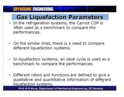
So now, we will come to the imported cycles. Before we go into various liquefaction cycles, let us find out what the different gas liquefaction parameters are. So, we have got different cycles, and if I were to compare to this different cycles, I will have to compare different parameters. What are these parameters? In the refrigeration system, for example, the Carnot COP is often used as a benchmark to compare the performances.
