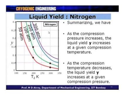
If I now extend this further, for different pressures, what you get is this at 200 atmospheres; and this at 300 atmospheres. It is fair to say that I should go for as high pressure as possible, and as low temperature as possible for the compression process.
