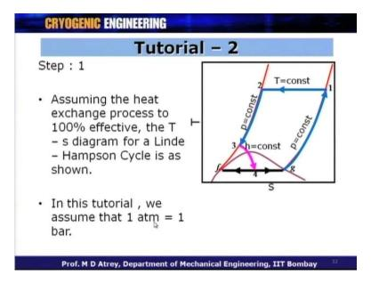
So, step one, as I said, the assumption is that, the heat exchanger is effective; 100% effectiveness. The T - s diagram from Linde - Hampson cycle is as shown. What is
