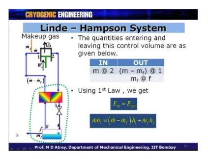
The quantities entering and leaving the control volume are as given below. What is entering is only the gas which is coming at m dot 2, the mass of gas which is coming at point 2, while, what is leaving the system is m minus m f dot, at this point. At the same time, what is leaving the system is the m dot f figure.
