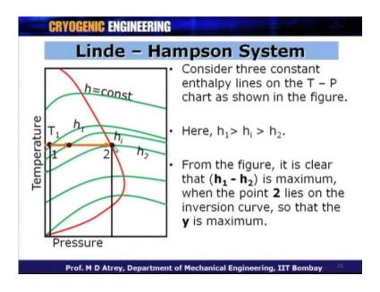
What do you understand from this? If you see at (() curve, which is the temperature, pressure diagram, and this is your inversion curve, and there are different enthalpy lines. If I want to compress the gas from point 1 to point 2 isothermally, that means, the temperature remaining constant, you can understand from here that, I can have various infinite values of different enthalpies, but my h 1 minus h 2 is going to be maximum only when the point 2 lies on the inversion curve.
