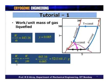
Now, the third requirement of the problem is to calculate the work required per unit mass of the gas, which is liquefied. What we calculated earlier, is work per unit mass of gas which is compressed. So, what we have earlier found is minus w c upon m dot is equal to 443.16 joule per gram.
