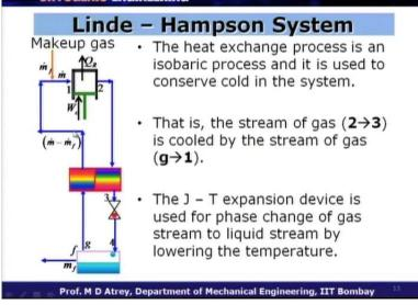
The heat exchanger process is an isobaric process, and it is used to conserve cold in the system; that means, when both the fluids are travelling through the heat exchanger, there is no pressure drop across the heat exchanger. That is, the stream 2 to 3, and g to 1- these points are the direction of the fluids flowing through here, the stream of the gas 2 to 3 is cooled by the stream of the gas going back.
