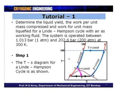
Let us have a small tutorial of one or two lectures. Under the first Tutorial now, the problem statement is, 'determine the liquid yield, which is nothing but y, the work per unit mass of gas compressed, which is nothing but W c upon m dot, and the work for unit mass of gas liquefied, which is nothing but w upon m dot f, for a Linde - Hampson cycle with air as working fluid'. It is very important to understand what has been asked in the problem.
