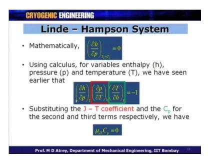
Mathematically I will say that, del h by del p, at temperature T 1, is equal to T 2, at point 1 is equal to point 2, this should be equal to 0. So, I get the minimum value of h2 here, or I get maximum value of h 1 minus h 2, in that case.
