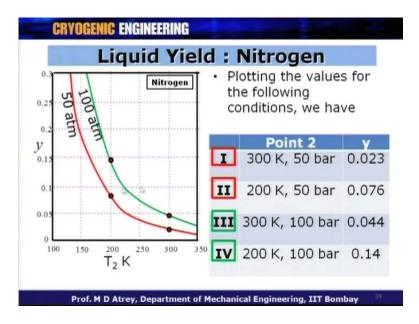
If I want to plot this now on y as a function of T2 that means, the compression temperature, or the isothermal compression temperature you can see is, point number 1. This point 2, if I plot at 200 Kelvin and 50 bar pressure is this; and if I join this point and extend this point further, this is the line of 50 atmospheres, and you can see as you go on loading the temperature of the compression, the yield is going to increase in this fashion.
