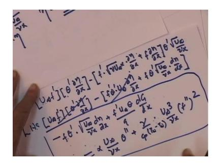
Remember, if I were to replace this n by n nu x U infinity by nu x, then you will see that I get U infinity f dash into theta dash d eta by dx minus f dash. n is equal to under root nu U infinity x d eta by dx plus f dn by dx into theta prime under root U infinity by nu x. Therefore, you will see this becomes U infinity f dash into theta dash d eta by dx minus f dash into theta dash U infinity d eta by dx plus f theta prime under root U infinity by nu x dn by dx.
