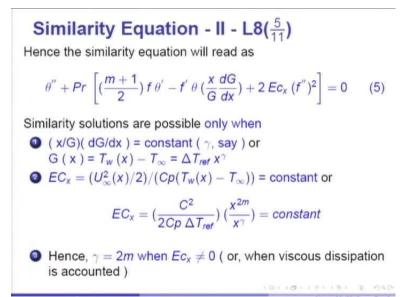
Remember similarity solutions to the temperature boundary layer are possible when Ec is ignored - that is viscous dissipation is ignored. Then, gamma can take absolutely arbitrary values. But, when viscous dissipation is included, gamma can take only restrictive values - gamma equal to 2m.
