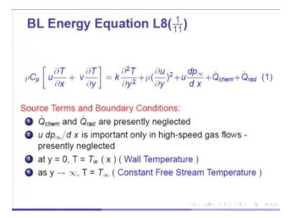
Therefore, upon substitution, you will see the equation would become dividing through by rho C p, I will get u dt by dx plus v dT by dy equal to alpha d2T dy square plus mu by rho C p du by dy square. If I substitute these three derivatives here, I will get T w minus T infinity into u d theta by dx plus v d theta by dy plus theta into u dT w by dx equal to alpha into T w minus T infinity into d2 theta by dy square plus nu by C p du by dy whole square. That is what I will get.
