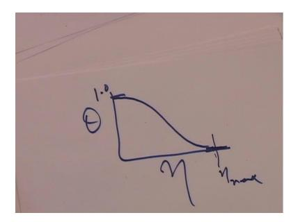
The physical thickness, delta is - remember our solution will look like this - theta verses eta, at wall it will be 1 and we expect the solution to go something like this with this 0 boundary condition at eta equal to some eta max. So, how do we choose the value of the thermal boundary layer thickness?
