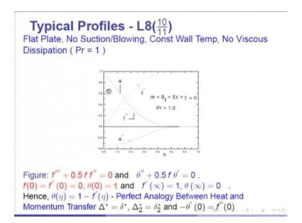
So, you will see here the earlier solution, f for f dash - this is a velocity boundary layer equation for Prandtl equal to 1 and the boundary layer thickness for the velocity was about 5. Likewise, the temperature profile theta should be 1 minus f dash eta. So, theta is nothing but - 1 minus f dash eta. This is the f double prime 0 which is going. Here, it is the theta double prime theta double prime or theta prime at x equal to 0.
