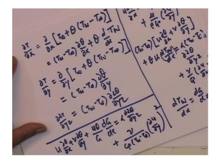
Notice dT w by dx is nothing but dG by dx. T w minus T infinity is nothing but G. Therefore, if I divide through by G, I will get u d theta by dx plus v d theta by dy plus u theta by G dG by dx equal to alpha times d2 theta by dy square plus nu by Cp T w minus T infinity du by dy whole square.
