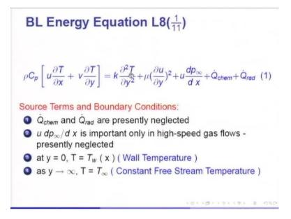
And eta as you will recall equals y into under root U infinity by nu x. If I make the substitutions of these two quantities in the differential equation, you will notice that I am going to replace T in these three terms by theta.
