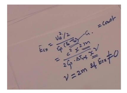
Ec x is U infinity squared by 2 divided by C p into T w minus T infinity and this is equal to c squared x raise to 2m divided by 2 times C p - and this is - delta T ref x raised to gamma. G is T w minus T f. Therefore, Ec x will be constant, if this is constant then this and this must cancel which means gamma must equal 2m, if Ec x is not equal to 0.
