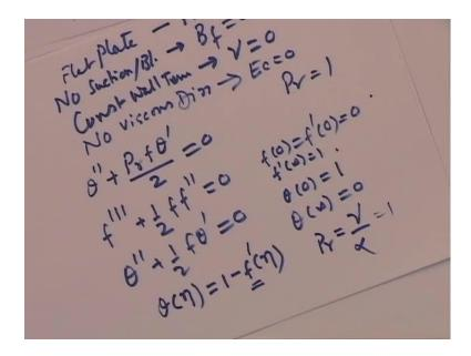
Flat plate means - m equal to 0; no suction blowing means - B f is equal to 0; constant wall temperatures means gamma is equal to 0; no viscous dissipation - means Ec is equal to 0.
