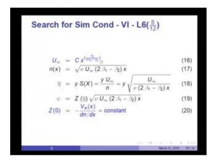
If I integrate this (Refer Slide Time: 22:27), it gives me the first similarity condition that U infinity must vary as C x raise to beta 2 over to beta 1 minus beta 2. If I integrate this from 0 to x, you will see (Refer Slide Time: 22:45) ln U infinity will be constant times ln X and therefore, the relationship follows. So, ln U infinity equal to same constant ln X or U infinity would be constant times C x raise to beta 2 over 2 beta 1 minus beta 2.
