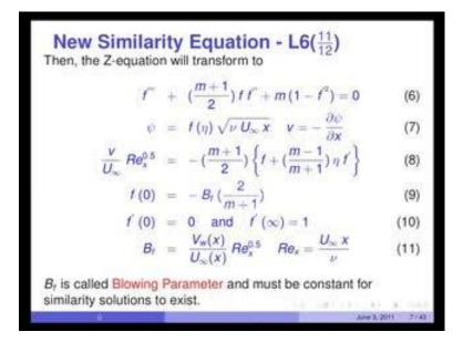
You will now get a solution to v in terms of f, f dash and eta. So, v is a function of eta is known in terms of the pressure gradient parameter m. At f 0, you have V w by dn by dx so that it will transform into V w x by U infinity Re x by because all I do is if f equal to 0, I have simply put f 0 and f dash 0. f dash 0 is 0 already; as you now, will become the no slip condition.
