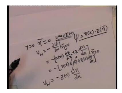
What are the boundary conditions? First of all, at y equal to 0, eta bar equal to 0, I have u equal to 0 or that will be equal to Z prime 0; that is, the no slip condition, which I have mentioned here.
