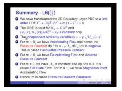
Let me summarize. We have transformed the 2D Boundary Layer partial differential equation to a third order ordinary differential equation f triple prime plus m plus 1 half f f double prime plus m 1 minus f double prime square equal to 0.
