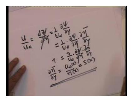
We will recall that u over U infinity as I defined is dz by d eta bar and that is equal to 1 over U infinity into d psi by dy. However, notice that I can write this as 1 over U infinity d psi by d eta bar into d eta bar by dy, which I can write as...
