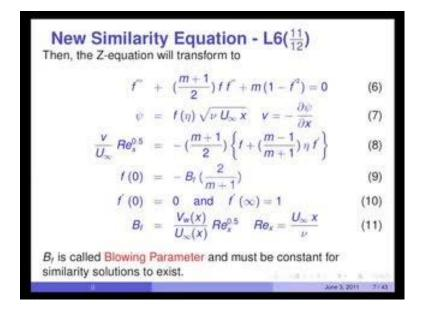
In the new similarity variable f and eta, appropriate Z equation will transform to this equation in f. psi is equal to f eta under root nu U infinity x and therefore, v will be equal to d psi by dx.
