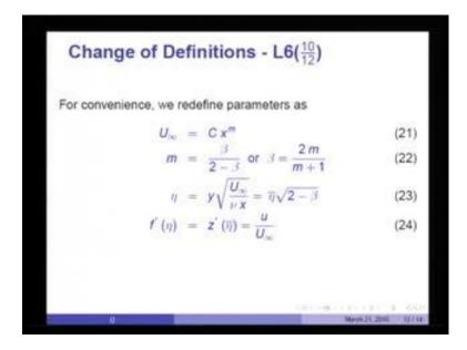
Having to write beta over 2 minus beta every time makes life somewhat difficult. So, I have simply defined m equal to beta over to 2 minus beta or beta is equal to 2 m divided by m plus 1. I have simplified eta by removing 2 minus beta into it. Now, the new variable is eta, I am replacing z by f and saying f dash eta will be equal to z dash eta bar equal to u over U infinity, as before.
