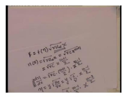
If you differentiate this equation, you will see psi equal to f eta under root nu U infinity x, which is really the n x. So, n x is equal to under root nu U infinity x, but U infinity is c x raise to m. Therefore, nu c x raise to m plus 1. That will be equal to nu c x raise to m plus 1 by 2. dn by dx will be under root nu c into m plus 1 by 2 into x raise to m minus 1
