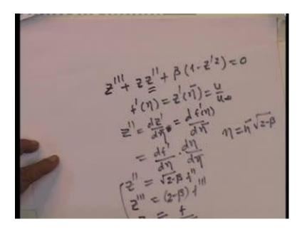
With this substitution, then you will notice that our equation Z triple prime plus Z Z double prime plus beta into 1 minus Z prime square equal to 0 and I am changing this. Remember: I have said f dash eta equal to Z dash eta bar equal to u over U infinity.
