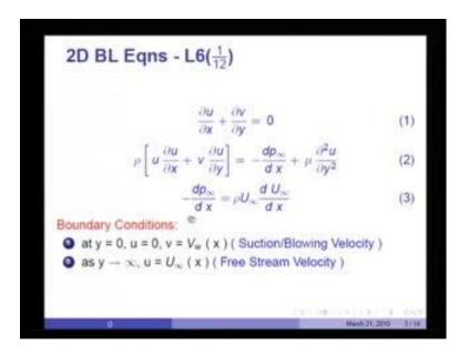
Let us recall the equations. The equation is the so-called mass conservation or the continuity equation for a constant property steady flow, du by dx plus dv by dy equal to 0. These are the convection terms in the momentum equations – the pressure gradient and the viscosity effected term, mu d 2 u dy square. We said that if this equation was written in the infinity state, then the pressure gradient could actually be written as rho U infinity d U infinity by d x.
