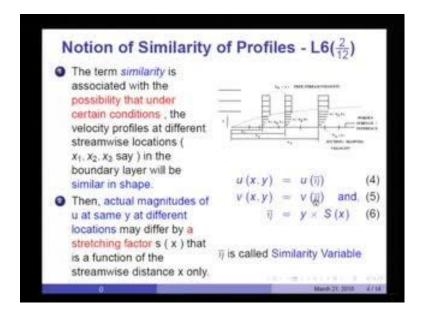
What is the notion of similarity profiles? The term similarity is associated with the possibility that under certain conditions the velocity profiles at different stream-wise locations, x 1, x 2, x 3, say in the boundary layer will be similar in shape.
