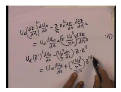
As a result, then I would have the equation, which would look like this; U infinity U infinity into dz by d eta bar whole square (Refer Slide Time: 16:36) into d U infinity by dx would be the first term; that is what I have written here (Refer Slide Time: 16:41).
