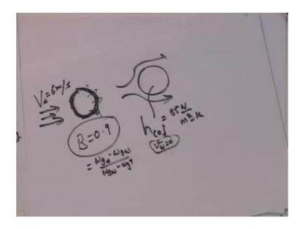
We now take up a problem, benzene evaporates from the outer surface of a circular cylinder, so let us say I have a circular cylinder like this on which a benzene has been put, and there is a cross flow across the across the cylinder, and therefore the benzene evaporates, the approach velocity v infinity is 6 meters per second.
