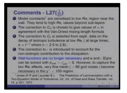
Now, in the early path at small times the kinetic energy decays again as t raise to minus n, but n would be then of the order of 1.1 to 1.2, but at large times it becomes 2.5 to 2.8. C 2 is again determined exactly from the same procedure as before, but the value of C 2 is corrected as shown here; it is sensitized to turbulence Reynolds number.
