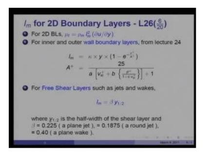
As I said y half is the half width of the shear layer and beta takes different values. This is been observed from experiments as well as has been tuned by numerical experiments. So, beta equal to 0.225, if the jet was a plain jet; if it was a round jet, it would be 0.1875 and if it will a plain wake, it would be 0.4. So, these are the typical values for free shear
