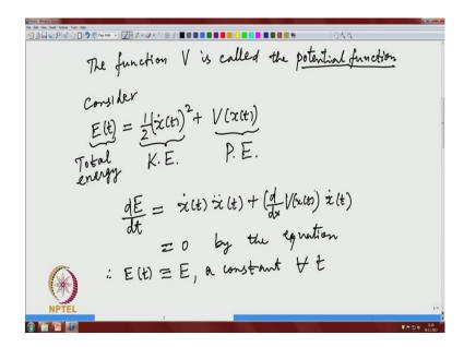
The function V is called the potential function. The terminology again comes from classical mechanics. So, consider this quantity. So, if x is a solution of that conservative second order equation. Consider this quantity x dot t square plus V x of the, and using, so if. So, let me call this as E t, E of t. So, x t is a solution of that equation. So, this represents kinetic energy and this represents potential energy. So, this is the total energy at time t, total energy of the particle.
