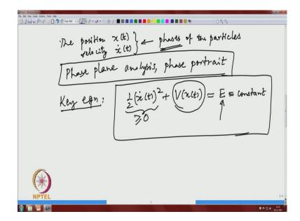
So, and the position x t and velocity x dot t, these are called as phases of the particle. Again, terminology comes from mechanics. So, we will do analysis involving phases that is phase plane analysis. And when you describe the position and velocity for all time and that is described as phase portrait. So, that is phase plane analysis, these are the terminology coming from this. This plane because there is only position and velocity.
