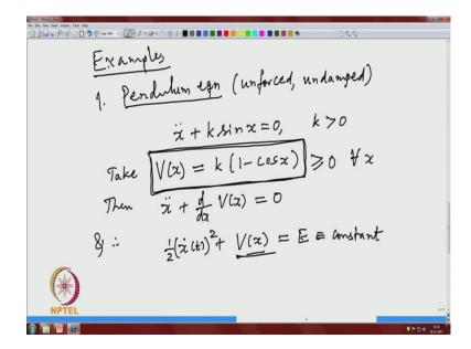
So, we are not adding any force. So, this is unforced and there is no damping. So, this is un-damped. So, this is the equation x double dot plus k sin x is equal to 0. So, k is some fixed constant, k is a positive constant. So, this can be written as a conservative equation so by. So, take there are many choices and I will explain by this particular choice. So, this you take V x is equal to k into 1 minus.
