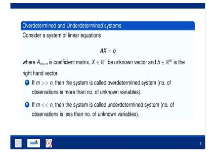
So, consider a linear system of equations A X equals to b, where A is m by n coefficient matrix, X is the unknown vector belongs to R n and b belongs to R m is the right hand side vector, which is given to us.
