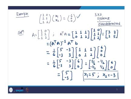
So, let us take example. So, what I am having  $1 \ 0 \ 1 \ 1 \ 1 \ 2$ , into x 1 x 2 equals to 6 0 0. So, it is a 3 by 2 system, means three equations in two unknowns x 1 and x 2. So, it is an over determined system.
