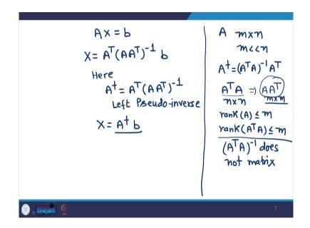
So, what I am having a system A X equals to b. Here A is m by n matrix and m is less than n. In the case of least square approximation you have seen that pseudo inverse is A transpose A inverse into A transpose.
