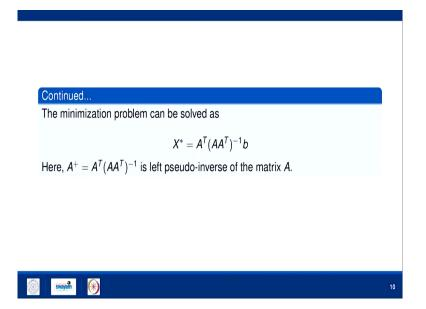
Here we will calculate the pseudo inverse is. So, instead of A transpose A, I will go for A A transpose, which is again m by m matrix. And if the rank of A transpose A A T is m then what I will be having, I will be having this as a full rank matrix so inverse exists and I will use this concept.
