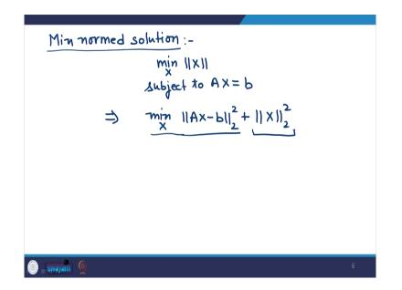
So, mathematically how can we pause this problem? So, we have to find out X, which minimize the norm of X, subject to A X equals to b. So, A X equals to b that it should be a solution of this linear system, this linear system will be having infinitely solution. So, out of those infinite solutions I am interested in the solution which is having the minimum norm.
