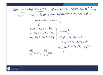
So, least square approximation. So, given A X equals to b, where A belongs to R m by n, that is A is m by n matrix having real m (Refer Time: 10:12). And m is quite bigger than n that we are having an over determined system. So, in this case, how to find out least square approximation?.
