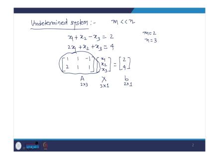
If we talk about underdetermined system then what we are having. So, in underdetermined system we are having, that is the less number of rows than the unknown variables. So, for example, we are having some system like this x 1 plus x 2 minus x 3 equals to 2 and 2 x 1 plus x 2 plus x 3 equals to 4.
