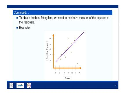
So, what is residual? The directed distance between the observed data points and the corresponding points on the model line is called the residual. And then sum of the square of all those residual is called the residual error. So, just see this example, here we are having this tenure that is in months and here monthly charge. And we are having in 2 dimensional plane these data points, so certain data points.
