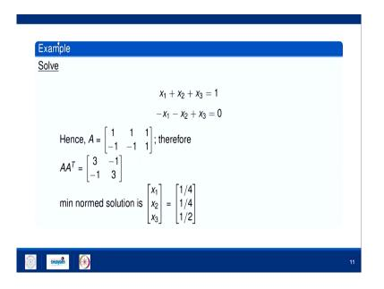
So, let us take an example of this. So, example is  $x \ 1$  plus  $x \ 2$  plus  $x \ 3$  equals to 1. And another equation is minus  $x \ 1$  minus  $x \ 2$  plus  $x \ 3$  equals to 0. So, it is an underdetermined system because we are having three unknown variables  $x \ 1$ ,  $x \ 2$  and  $x \ 3$  and only two equations. So, this system will be having infinitely much solution.
