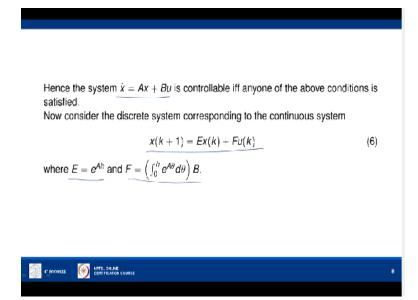
So the system, continuous system is x dot=Ax+Bu and the corresponding discrete system is x of k+1=E\*x of k+F\*u of k where e is given by this expression as we have seen earlier and F is given by this. The A and Bare constant matrices.
