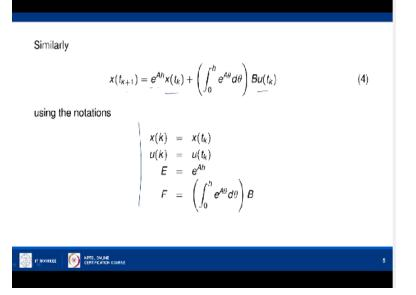
So now if we proceed in the similar way, we get x of tk+1 is e power th\*x of tk + integral 0 to the power A theta d theta\*this. Now if we use this notation x of k is x of t suffix k and u of k is u of t suffix k, e is the matrix given here, e to the power Ah and F is the matrix given in this second term, integral 0 to the power A theta d theta\*the matrix B.
