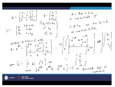
So if you assume that the matrix A is given by this lambda 1 is the eigenvalue and lambda 2, so let us say lambda 1 is not equal to lambda 2 and it is in the Jordan canonical form like this and the matrix b is a column vector b1 b2 b3. So in this case, the system x dot=Ax+Bu is controllable if we have b, b is the column vector, b1, b2, b3. A\*b that gives lambda 1b1+b2 and second is lambda 1\*b2, then lambda 2\*b3.
