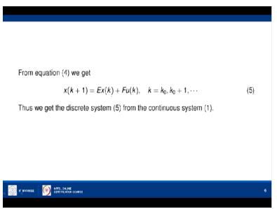
So if this matrix is F, then by substituting these in the equation 4, we get the corresponding discrete system that is x of k+1 is ex of k+Fu of k, k is ranging from k0, k0+1, etc. So from the continuous system 1 getting the discrete system 5 here. So now can we use this discrete system for all purpose that is the controllability, observability, stability of system I, can we apply it to the system 5 as it is?
