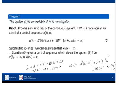
So the theorem analogous to the continuous case is, the system 1 is controllable if and only if the controllability Gramian matrix W is nonsingular. So the proof is similar again to the continuous case. Earlier, we defined the case, in the continuous case we define u of t to be=B dashed of t phi dashed t0, t\*the Gramian matrix for continuous case, its inverse\*phi of t0 and final time\*x1-x0 the initial condition of the system.
