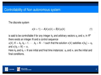
So let us consider the time varying system x of k+1=A of k x of k+B of k u of k as given in equation 1. So the system is said to be controllable if for any initial integer k0 and arbitrary vectors x0 and x1 in Rn the state space there exists an integer N that is final instant and a control sequence u of k0, u of k0+1, etc u of k0+n-1 such that the solution of 1 satisfies x of k0 is the initial condition given x0 and x of k0+N is x1 the final condition.
