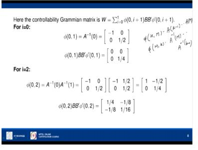
So if you directly apply the formula, the controllability Gramian is summation i ranges from 0 to k N-1 so that is 2-1, it starts from 0 and end with 1 phi of k0, i+1 BB dashed phi dashed 0, i+1 that is k0 is 0. Now we can calculate by recalling phi of k, M it means A of k-1 up to A of M. So when we take and similarly phi of M, k we have seen that it is A inverse of M, etc up to A inverse of k-1.
