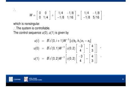
So summing these two we get the controllability Gramian matrix given by this expression and can be easily verified that it is nonsingular. So according to the theorem, the system is controllable. So the control variable which we want to find is given by this expression. We have seen the formula in 5 is one control which will steer the system from initial x0 to the final condition x1.
