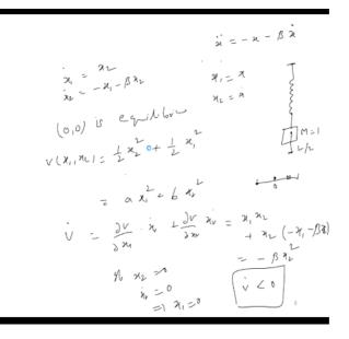
So now we consider a system like this. For example, x1 dot=x2, x2 dot=-x1-beta times x2. So this system it is nothing but a harmonic oscillator type of thing, x double dot=-x-beta times x dot. So this is either you can consider this as a mechanical system where the mass=1, mass\*acceleration that is the left hand side that is the force and it is due to the spring constant. Here we are assuming the spring constant=1.
