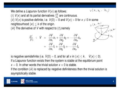
So if you are able to find a Lyapunov function V of x, here we note that x is a vector, this x is say x1, x2, xn belonging to belongs to Rn and f is also a vector, f of x means f1 of x, f2 of x, fn of x, so the nonlinear system of differential equations here. So when we talk about V of x, it means V of x1, x2, xn a function of n variable. So this function V of x and its partial derivatives are continuous function means continuous functions of this n variable.
