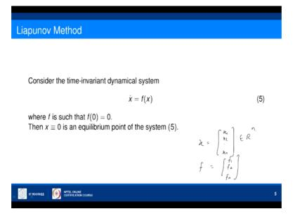
So in situations where the system cannot be stabilizable using this procedure, then we may try some Lyapunov method for stabilizing a system. So first we will see a system which is not having any control term, simply a nonlinear term and time invariant that is autonomous system x dot=f of x where f is either linear function or some nonlinear function such that f of 0 is 0. So that will imply that x=0 is the equilibrium point for the system 5.
