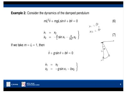
So now we will consider examples in which the Lyapunov function need not be in the form of an energy function. So let us consider the system mL square theta double dot+mg L sin theta+b theta dot=0. So this is a damped pendulum problem. So we have already seen this example. We have a pendulum of this type which is oscillating and this is the theta value. So we can write the equation where L is the length and m is the mass here and g represent the gravity.
