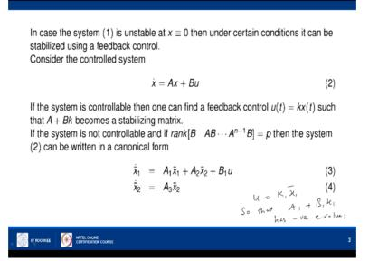
So in case the system is unstable at the trivial solution x=0, then we have also seen in previous lectures on feedback control that the system can be stabilized. We can find a feedback control u suitably so that the resulting system x dot=Ax+Bu becomes either stable or asymptotically stable depending on the requirement of the system. So this has been described in the feedback lecture with some examples also how to find the u of t=k\*x of t.
