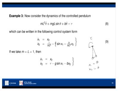
But if you want to stop this system at some other position let us say we want to apply a control on the pendulum. So the natural oscillation is due to gravity but if you apply a torque at this joint here, so that rotational force that is torque here can control the movement of the pendulum. So that is called the controlled pendulum and we can write the system equation as in the same manner x1 is theta and x2 is theta dot.
