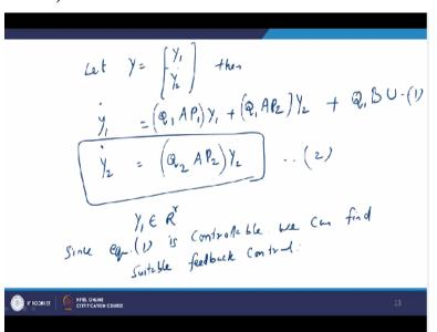
So if we write y to be, it is an Rn vector. We will write it as y1 vector and y2 vector, first R elements are called y1. The remaining n-r elements are called y2. So if you write like this, then we get from the previous page, we will get y1 dot, the derivative of y1 is Q1AP1\*y1+Q1AP2\*y2+, here Q1B\*U vector we will get, okay. Similarly, y2 dot will be 0\*y1, so that will not come.
