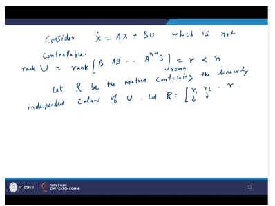
And now we will reduce the non-controllable system into a system which has 2 parts. One portion is controllable portion. Another portion is non-controllable portion. And then we can apply the same theorem for one portion that is which is controllable portion, okay. So consider the system X dot=Ax+Bu which is not controllable. So that means the rank of the matrix, the block, first block is B, second block AB, and A power n-1B, this rank is equal to, let us say r which is less than n.
