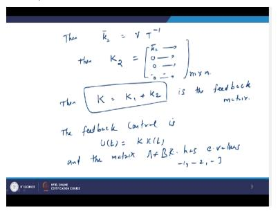
So from this calculation, we will get, finally we get then again recall the method which we have seen in the second lecture that is gamma\*T inverse, the row vector K is given by gamma\*T inverse. So once we calculate this, then we can calculate the K2 vector which we require actually. This procedure, we are defining this K2 vector where K2 vector is the first row is the matrix which we found and all the other rows are 0.
