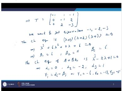
So that implies that T matrix is calculated as  $-1 \ 1 \ -1$  and  $0 \ -1 \ 2$  and  $0 \ 2 \ -3$ . After substituting the proper values in T matrix, we get this one. Now we want to find this feedback control for this expression that is we want to find the K2 matrix so that we ultimately find K1+K2. So for finding K2, we adopt the following procedure. So we are interested in getting, we want to get eigenvalues  $-1 \ -2 \ -3$  for the converted system.
