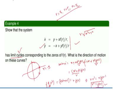
So, we can say that zero is a trivial limit cycle which is unstable limit cycle. Now, next example is a generalisation of the previous example showed that the system x dash = y + x + fr upon r, y dash = -x + y fr upon r, where r = x square + y square under root has limit cycle corresponding to the zeros of, f of r and what is the direction of motion of these curves that we wanted to find out so, if we look at how we look at so, xx dash + yy dash, if you want to find out.
