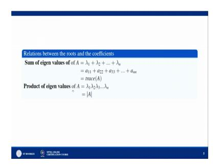
So, the sum of the eigen values simply equal the trace of the matrix. And the product of the eigen values simply the determinant of A.
