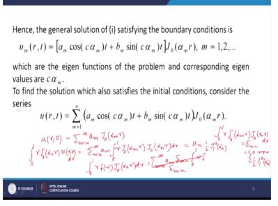
And what we do is that this is putting t=0 ur=0=sigma m=1 to infinity am times J0 alpha mr then we multiply both sides with r times J0 alpha n r and then integrate with respect to r over the interval 0 to 1 okay. So u r, 0 is given to be=f r, u r, 0 is given to be f r so let us put its value there and we will get it as 0 to 1 r f r J0 alpha nr dr=summation m=0 to infinity, now am here we have integral 0 to 1 r J0 alpha mr J0 alpha nr.
