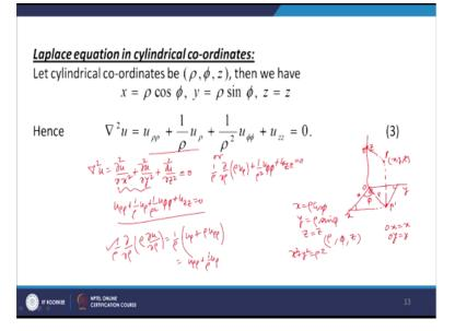
So we have to solve the equation, we can write this equation you can see we can write this equation also as 1/rho if I multiply the partial derivative of u rho with respect to rho and multiply 1/rho then what do we get, this is = 1/rho times derivative of rho with respect to rho is 1 so we get u rho and then we get rho u rho rho. So what we get here u rho rho+1/rho u rho.
