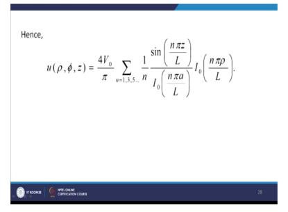
And this leads to the solution u rho, phi, z=4V0/pi where n runs over odd integral values\*1/n sin n pi z/I0 n pi a/L\*I0 n pi rho/L. So this is an example on the cylindrical polar coordinates, when we convert the Laplace equation into cylindrical polar coordinates. In the next lecture, we shall consider spherical polar coordinates and will solve Laplace equation in spherical polar coordinates. Thank you very much for your attention.
