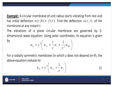
Let us take up the case of a circular membrane of unit radius starts vibrating from rest and has initial deflection u r, 0=f r. We have to find the deflection u r, t of the membrane at any instant t. Now the vibrations of a plane circular membrane are governed by 2-dimensional wave equation. Using polar coordinates as you know, its equation is given by u tt=c square u rr+1/r ur+1/r square u theta theta.
