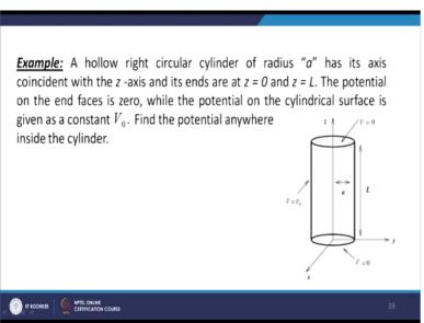
Now let us consider a hollow right circular cylinder of radius a which has its axis as coincident with z-axis and its ends are at z=0 and z=L this is z=L, this is z=0, the potential on the end surface is 0, potential on this face V=0 potential on this face V=0 and potential on this cylindrical surface is given as a constant V0, on this curved surface potential is given as V0. Now we have to find the potential anywhere inside the cylinder.
