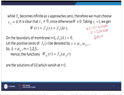
Now u 1, t=W1\*G t and W1=J0 k\*G t, so either J0 k is 0 or G t=0 if G t=0 then u r, t will be 0 so trivial solution we will have and therefore we must take J0 k=0 and J0 k=0 means the 0 is of the valid Bessel function of order 0. So let the positive 0s of J0 s be denoted by s=alpha 1, alpha 2 and so on so then k=alpha m where m=1, 2, 3, and so on. Hence, the functions Wm r=J0 alpha m r, for each value of the root of J0 s=0 we will have a Wr function.
