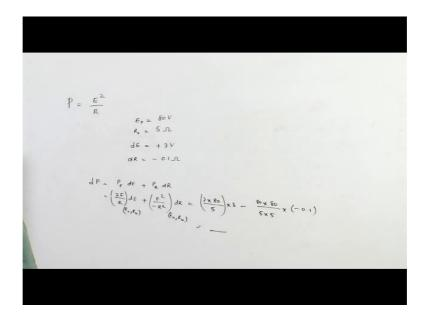
If e equal to 80 volt, and r equals to 5 ohms, how much power consumption will change if E is increased by 3 volt and R is decrees by 0.1 ohm?
