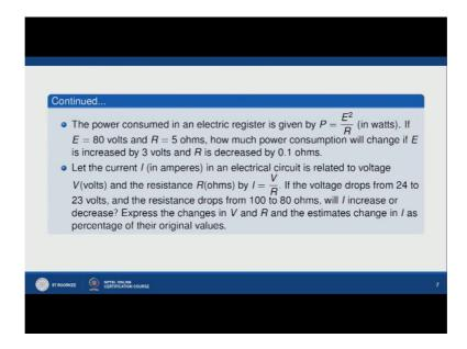
The power consumed in the electric resistance given by P is equals to E square upon R in watts.
