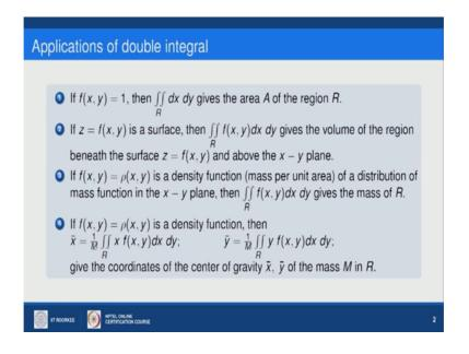
Double integral over R x times f of x y dx dy and y bar equals to 1 upon M double integral over region R y times f of x y dx dy gives the coordinates of the center of gravity that is x bar y bar of the mass M in R. If f of x y is rho, x y is a density function, then I x equals to double integral over the region R y square f of x y dx dy, and I y equals to double integral over R x square f of x y dx dy, give the moment of inertia of the mass in R about the x axis.
