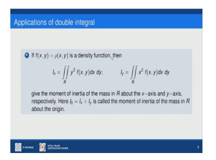
So, this is about x axis, and about the y axis this one. If I 0 is I x plus I y, then we say that moment of inertia of the mass R about the origin.
