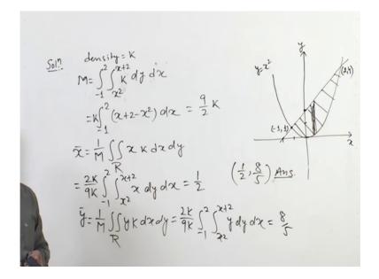
So, 2-dimensional region, whose density is constant, let us say k and is bounded by the curve y equals to x square and y equals to x plus 2. So, the plate is like this x y. So, y equals to x square, and the other one is y equals to x plus 2. So, it will cut 1 2, 1 2. So, the region is this one. So, we have to find out the moment of inertia of this plate when the density is constant. So, it will intersect at this point; which will be minus 1 and 1 and this point will become 2 and 4.
