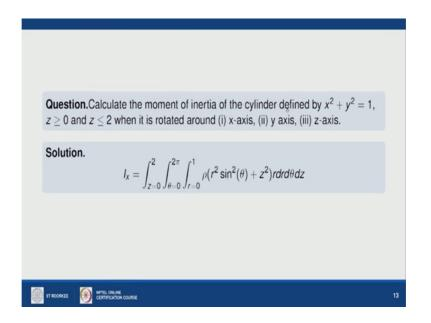
So, moment of inertia about x axis I x is given by; so, z is given 0 to 2. Now x square plus y square equals to 1. So, this is the cylinder of radius 1 along z axis. So, on the xy plane the projection of this cylinder will be circle of unit radius. So, we can change it in 2 polar coordinates so, theta will move from 0 to 2 pi and r will move from 0 to 1 rho r square sin square theta plus z square r dr d theta dz.
