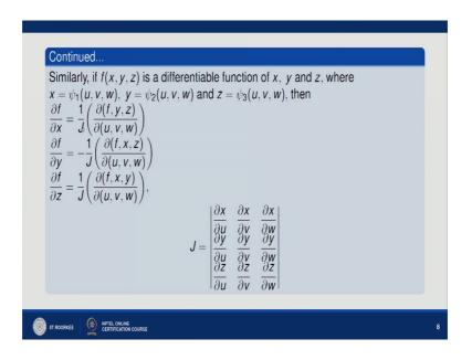
So, f x we can obtain as 1 by J times del of f y z upon del of u v w. Similarly, del f upon del y and del f upon del z; where J is simply del of x y z upon del of u v w.
