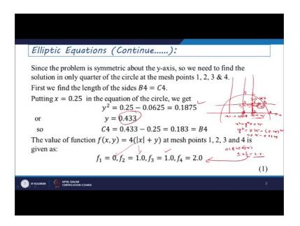
This problem is symmetric about y axis. So, we need to have to find the solution in the quarter of the circle, at the mesh points if you will just see here that is at a 1 2 3 4. So, this point, this point, this point and this point here.
