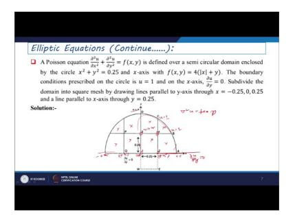
We are just considering here this problem which is like semicircular domain or irregular grid points can be chosen to find the solution. So, for this position equation the problem is given like a del square u by del x square, plus del square u by del y square this equals to f of xy is defined over a semicircular domain enclosed by the circle x square plus y square this equals to 0.25 and x axis with f of xy equals to 4 into mod of a x plus y.
