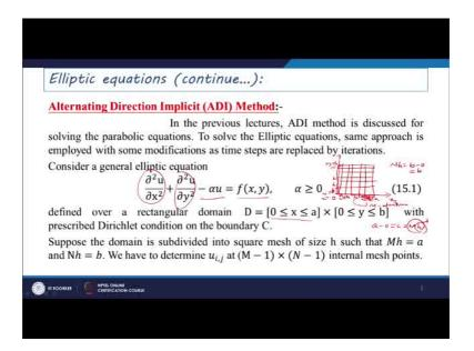
So, if you will just go for this ADI method here for a elliptic equation. So, alternating direction implicit method especially that is considers. So, this some of the steps calculation like in the x direction, we can just consider like a half step calculation and in the y direction we can just consider another half step calculation.
