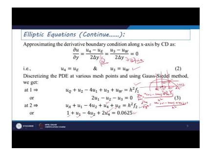
So, if you will just go for this derivative condition which is a defined at along the x axis here. So, we can just find that a del u by del y that is nothing, but this last point which is defined as a u 4. So, for this derivative condition if you will just see in the picture here we have just defined here like a fictitious domain there. So, this fictitious domain we are just giving this w as the west coordinate here and east part it is just written as a e here.
