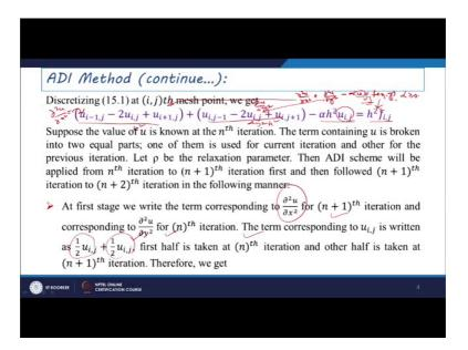
So, if you will just go for this discretization of this equation, that it is just represented here in the form like del square u by del x square, plus del square u by del y square minus alpha u, this equals to f of x y for alpha greater than equal to 0.
