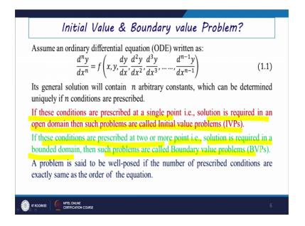
So, if we want to find the solution of this differential equations especially, if we will just integrate these differential equations then we can just find some constants there; to find the values of these constants especially we have to put either this initial condition or the boundary condition to get it free from these constants or independent solutions there.
