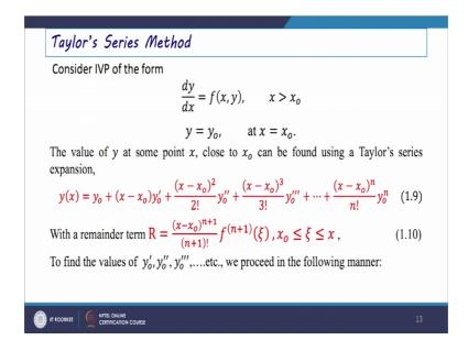
So, first we have to consider that if the function is defined at its initial point or at certain point close to that point this function should be continuous, if the function is continuous at the neighborhood point then we can just expand in Taylor series form. So, if you will
