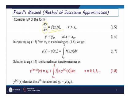
So, if you will just go further like how we can just use any numerical method for such class of like initial value problems. So, first method is we have considered here that is as Picard's method here that is especially called method of successive approximations.
