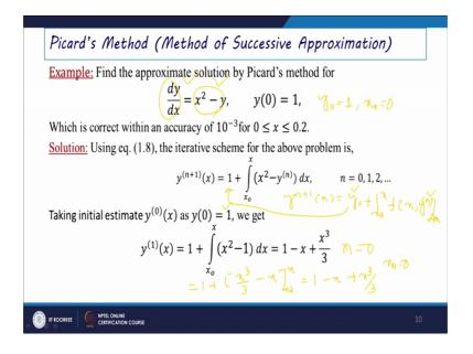
Especially I am just signifying this one this differential equation as a dy by dx that is the first order differential equation we can just say and this f of x y part it is just carrying like a x square minus y part here and the initial condition that is the given as y naught, we can just write here y naught equals to 1 when x naught equals to 0 here.
