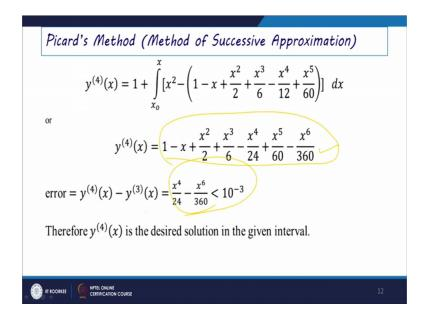
And if you will just go for this error computation at the same point that is as x equals to 0.2 then we can just find that this error is less than 10 to the power minus 3, hence we can just say that y 4 x is the desired solution within that given interval.
