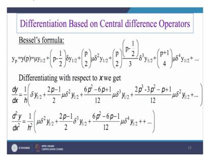
Similarly we can just use this formulation for like Bessel's formula here so Bessel's formula usually it is expressed as like y p = y of x p that as Mu y of half here so if you just write this one as y p in Bessel's formula here, this is for Stirling's formula here.
