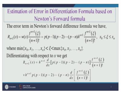
So if you will just go for this error term analysis based on this Newton's forward difference formula, so usually these error terms for this Newton's forward difference approximation is written in the form like  $R \, n + 1 \, x$  this = omega x f to the power n + 1 Zeta by n + 1 factorial, where this Omega x is usually written in the form like  $x - x \, 0$ , x - X1 to  $x - x \, n$  here.
