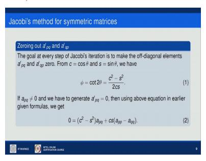
So if I make them zero, I can write zero equals to C square minus S square apq plus CS app minus aqq like this. Given by equation 2, moreover the goal of every step of Jacobi equation is to make the off diagonal elements a dash pq and a dash qp zero. So from this we can have phi equals to cot 2 theta C square minus S square. So it will be cos 2theta minus twice of cos theta into sin theta that is sin 2theta. So this is phi.
