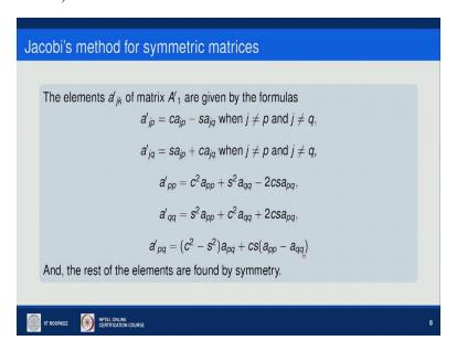
If we see this transformation in n by n set up, so what will be the relation between matrix A and A dash? So the elements said a jk of the matrix A dash are given by the formula. So when j not
