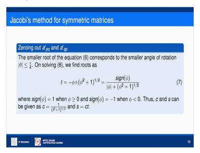
The roots of this quadratic equation is given by minus phi plus minus square root of phi square plus 1 and that will be sign of phi upon absolute value of phi plus square root of phi square plus . Here, sign of phi is 1, when phi is non-negative and it is minus 1, when phi is a negative number. Thus, once we get t we can calculate C and S by this formula C will be 1 sign upon square root of t square plus 1 and S will be C times t.
