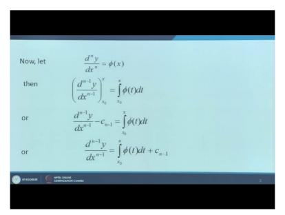
or we can say d n minus 1 y over d x n minus 1 is equal to integral x 0 to x phi t dt plus c n minus 1.
