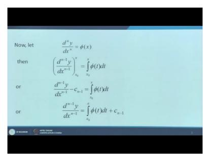
So let us see we will we start with let us define d n y over d x n equal to Phi(x). Then we integrate this with respect to x over the interval (x 0 to x).
