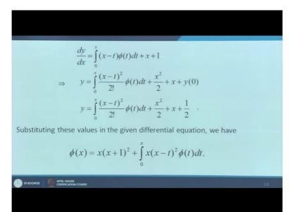
So we get Volterra Integral equation of the second kind. This x cube plus 2 x square plus x can be written as x times x square plus 2x plus 1 which is x times (x plus 1) whole square. So we get Volterra Integral equation of the second kind.
