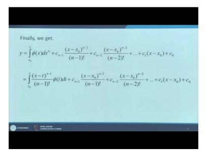
So after n integrals n times integrals taking integration n times we will get y equal to x 0 to x phi x d x n this means that n th derivative n integrals of phi(x) with respect to x over the interval x 0 to x plus c n minus 1 x minus x 0 to the power n minus 1 over n minus factorial
