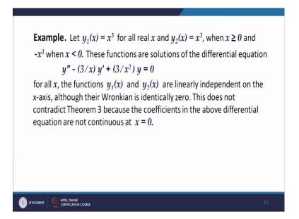
You can easily check that y 1 x equal to x cube satisfies this equation for all real x, and y 2 x equal to x cube when x greater than or equal to 0, and minus x cube when x less than 0; they also satisfy this second order differential equation for all x. So, both y 1 and y 2 are now moreover we can see that y 1 x is x cube, for ordial x while y 2 x is x cube when x is greater than or equal to 0, minus x cube when x is less than 0.
