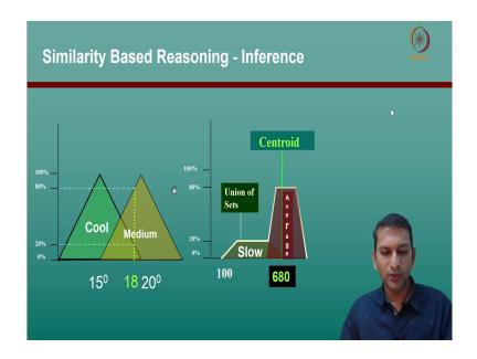
So, it is clear visually what we are doing is applying min, the min t norm as the modification function. So, that is the second step we have modified it. The third step involved taking the
