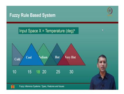
What we have? We have this partition on input domain. Let us assume 18 is the value that is given to us as input; that means, the sensor and the air conditioner sense it is 18 degree centigrade. Now, question is what should be the fan speed that is what we want to do. How do we do this?
