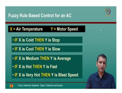
So, let us stay with this example of building a fuzzy controller for an air conditioner. So, we have identified that input is air temperature output is the motor speed and motor speed is what we want to control. By controlling the motor speed, we want to control the air temperature in the room.
