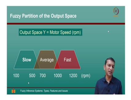
Next, the logical step is to partition the output space. The output space is Y which consist of motor speed. Let us assume that these are the motor speeds that we have in terms of rpm and for the moment let us have only 3 output fuzzy sets – fast, it should of course, looks look like this somewhere on the right extreme; slow which is looks left extreme and average.
