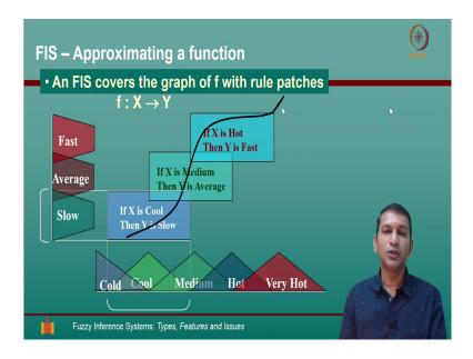
Now, the inferencing itself remember what we said was a fuzzy inference system approximates a function. What is that function? It captures the working of the system. So, there is some particular way in which an airs air conditioning control system should work, that is what we feel. If this is the temperature this should be the speed at which it should cool if this is the temperature.
