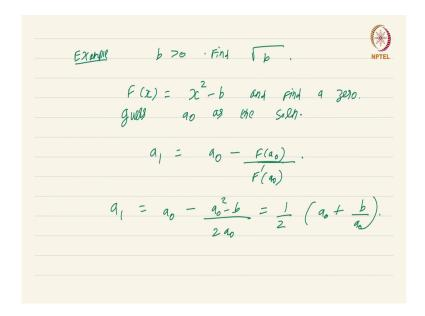
So, the example is as follows. We have b greater than 0, find square root of b, find square root of b, ok. So, what we are going to do is naturally to apply Newton's method. We are going to consider the function F of x equal to x squared minus b and find a 0. This is the aim, ok. So, of course, what does Newton's method say? Guess, a naught as the solution as the solution, ok.
