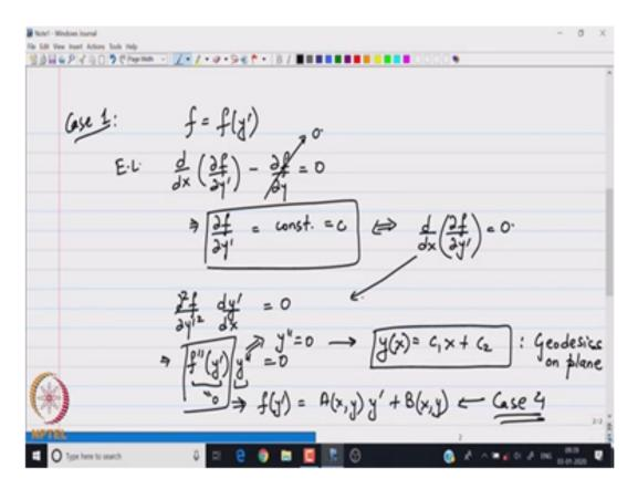
As I said, in the first case my f is only a function of y'. So by Euler equation  $\frac{d}{dx}\left(\frac{\partial f}{\partial y'}\right) - \frac{\partial f}{\partial y} = 0$ , we see that since f is not a function of y explicitly so  $\frac{\partial f}{\partial y} = 0$  and the equation shows that we can immediately integrate with respect to x
