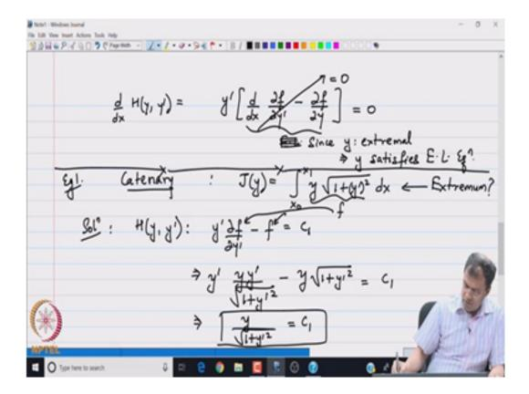
So, we can see the power of the result in this case. The Euler-Lagrange equation has reduced to H which is a first order differential equation as opposed to a second-order differential equation governed by Euler-Lagrange equation.
