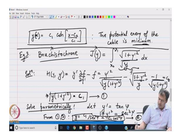
So, this is a much more convenient form of expressing the extremal in this particular case. And if we recall in this catenary problem, we are trying to minimize the potential energy of the cable.
