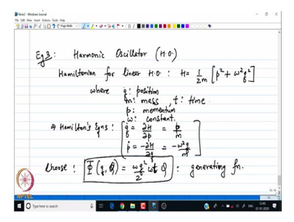
**Example 3** is of harmonic oscillator (H.O), the Hamiltonian for the linear harmonic oscillator is H given to be the sum of the kinetic energy plus the potential energy and I write it in terms of the conjugate variable p and q.
