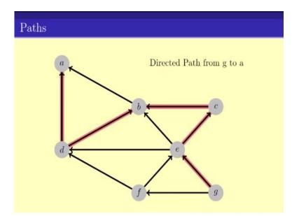
But if the graph is directed for example is this. In that case, as you can see this following the red path is not exactly a path because g, e is fine, we can have a path from g to e, a from e to c, c to b, but there is no edge from b to d. So this b to d is a problem. But there is a path from g to a in this graph, which is this one.
