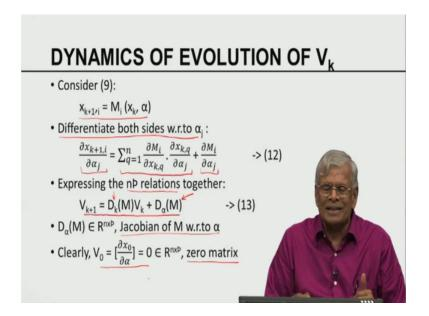
Now, we are going to concentrate on deriving a similar dynamics for V k. Please remember V k is the sensitivity the solution with respect to the parameters. Again I am going to consider the ith component of the model equation that was also the starting point previously. Earlier we found the derivative of this with respect to the jth component of the initial condition here we are going to differentiate this with the jth component of alpha.
