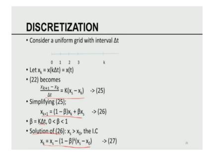
I am now going to discretize the model equation using standard Euler scheme this is the standard Euler scheme. So, if I simplify this 25 I get this equation. This is again a linear
