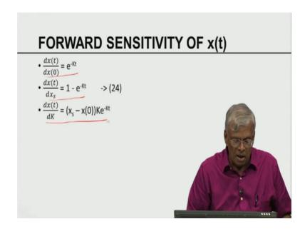
So, because the solution is known I can compute the sensitivities rather explicitly, I do not have to use the differential equation to compute the evolution of the sensitivity. So, that is the initial condition sensitivity, boundary condition sensitivity, parameter sensitivity.
