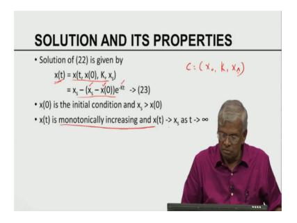
The solution of this model can be given explicitly because simply a first order differential equation we can readily solve from standard experience in calculus. So, this is the solution this is the form of the solution x naught is the, you can see the solution depends on x naught the solution depends on x s which is called the boundary condition and the solution also depends on the parameter x. So, the control here x consists of x naught, x and x s.
