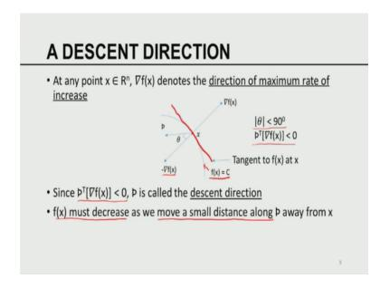
So, what is the basis for the gradient technique; the gradient technique rests on the concept of what is called a descent direction descent direction; means the direction in which the function increases decreases increasing mean ascent decreasing mean descent.
