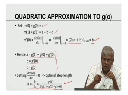
I can essentially estimate the parameters a b and c. So, m of 0 is g of 0 which is c m of one is g of 1 which is a plus b plus c m prime the derivative of at 0 is given by 2 a alpha plus b.
