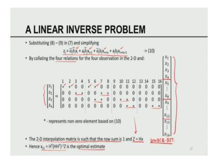
So, the right hand side has all the grid points z i j plus 1 j n n i plus 1 all the coefficients or distances that are known. So, I can write this in the form of a matrix. There are four observation, so there are four relations. So, this is the observation vector. There are 16
