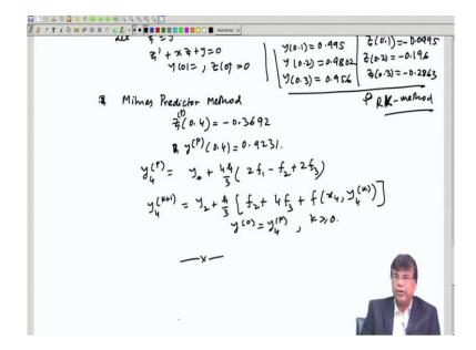
So, once we have these three points what is the precisely I wanted to say for this three we can use the Runge-Kutta method RK method and once we have that then the Milne's predictor corrector method for example this is more simpler than using the Runge-Kutta method and this is for professional computations for large time step solutions, this is the way one proceed. So, that is all about the IVP and next we will talk about the boundary value problem in the next class. Thank you.
