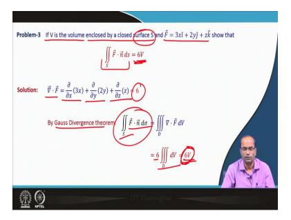
So, here we will see that if V is the volume enclosed by a closed surface S and this F is given by 3 times x, 2 times y and z times this K, then we will show that this flux integral F dot n ds is nothing but 6 times the volume of this surface. So here we will compute naturally we will apply the divergence theorem to see that how the 6 times V is coming and the idea is exactly from here.
