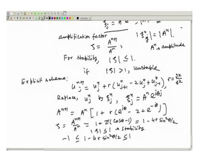
So, for stability we define another amplification factor that is I call as zeta is A n plus 1 by A n. Now, for stability what we require mod zeta should be less than equal to 1. So, if mod zeta is greater than 1 unstable. Now, obviously, the mod of xi n j is nothing, but xi n j is nothing, but mod of A n. So, this is A n is the amplitude. So, amplitude and theta is
