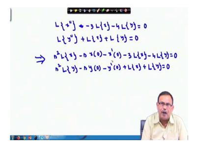
Basically instead of one equation, since now we have two simultaneous equations, we are applying Laplace transform on both sides of those two equations together. So, if we take the Laplace transform on both sides of the given equations, we will obtain,
