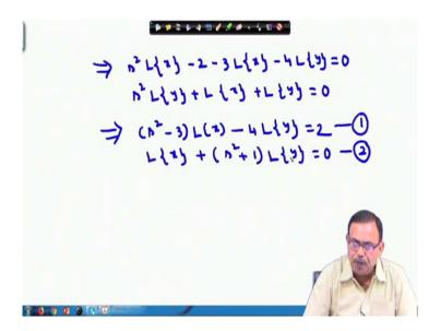
Therefore, we have basically two algebraic equations now in two variables namely,  $L{x}$  and  $L{y}$  which can be easily solved to obtain  $L{x}$  and  $L{y}$  separately as functions of *s*.
