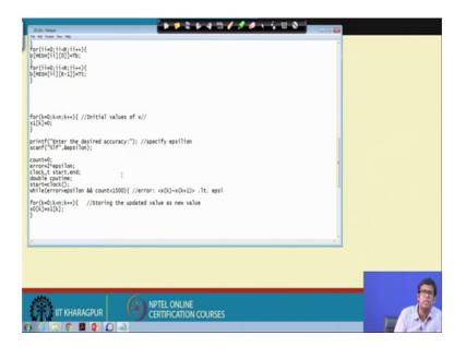
Then, we start with we have to give the desired value of accuracy which is epsilon that the user gives a gives it as a input and the program reads this value. The initial value is x
