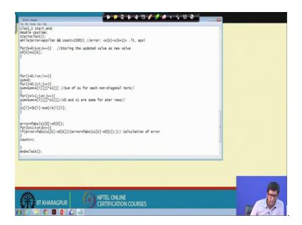
So, this is done for one particular  $x \ 1$  and similar and then, we calculate what is error what is the maximum value of  $x \ 1$  minus  $x \ 0$  for all the elements and check that check we will check what is the value of error and well like error is greater than epsilon, this loop will continue that means, count will be added by plus 1 and the control will be shifted here.
