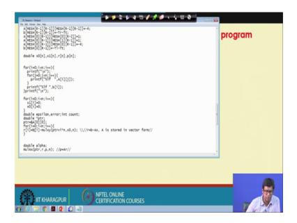
And then, r is equal to b minus multiplication of Ax; r is equal to b minus Ax and then we say it an accuracy epsilon. See this is for we start with the x is equal to 0 guess value and get r is equal to b minus Ax.
