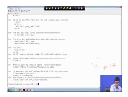
So, if I look into the Jacobi code, I have specified epsilon. I am not(Refer Time: 16:55) the epsilon from the user, but it is specified as 1 e 10 to the power the epsilon is specified as 1 e 10 to the power minus 8. So, if the value is less than 10 to the power minus 8, the iterations will be done.
