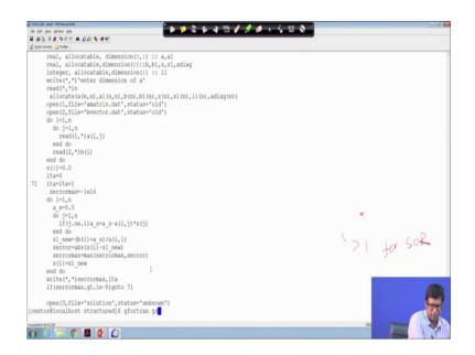
And now we do the same thing using a Gauss-Seidel and the iteration level is same. So, if I run the same code and this was 3000, more than 3000 steps.
