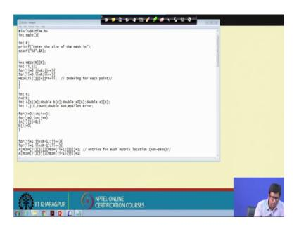
We are, so, what we are we have to here is that write down the initialize everything with the 0 and then, put the right boundary condition define the right coefficient of matrix A, it is inter diagonal matrix with the diagonal term minus 4 and all of diagonal 0 except few terms which are 1 and substitute the values of A for the boundary conditions and then, put the boundary conditions in the B matrix and so we get A and B fixed here.
