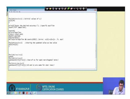
So and there is there are some comments for checking the computational time required for that. So, what you are doing here is that we are doing a sum for each sum of Ax for each non diagonal term until j is less than i. So, for all the non diagonal terms above the particular row is summed and this is total sum this is for one particular value of i. So, there is a loop over j; j is equal to i; j is equal to 0; j is less than i and there is another loop j is equal to i to j is less than n.
