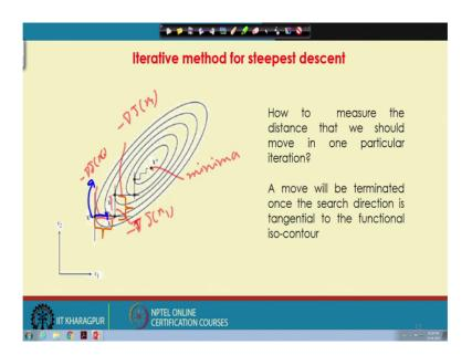
So, the method is pictorially like this. They start with one particular x 0 start with one particular x 0 move along a direction see it is being tangential to the functional here. Then you change the direction move along this find x 2. And so, this is this is like minus J x 0. This is like minus J minus gradient of J x 1 this direction this direction is minus gradient of J x 2 minus, you come to x 3 and change the direction and so on you approach the minimum value this is the minima.
