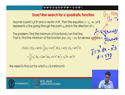
So, I have to find out the local minima of a function along a particular line. So, will first express the function along a particular line, how the function changes along the particular line. Assume a point x 0 which belongs to a real number coordinate of all dimension in rl and a vector y on that same space Rn. And then the equation y is equal
