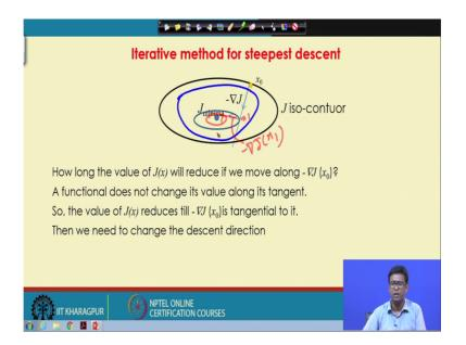
I have started with an x 0, how long the value of J x will reduce if we move along minus grad J evaluated at x 0. This I am moving along this minus grad J over this is evaluated at x 0.
