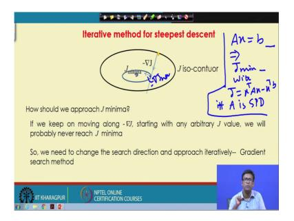
In steepest descent method what we have seen is that solving Ax is equal to b for an Ax is equal to b is equivalent to find out J minima with J is equal to x transpose Ax minus x transpose b and provided A is if and only if s symmetric positive definite matrix.
