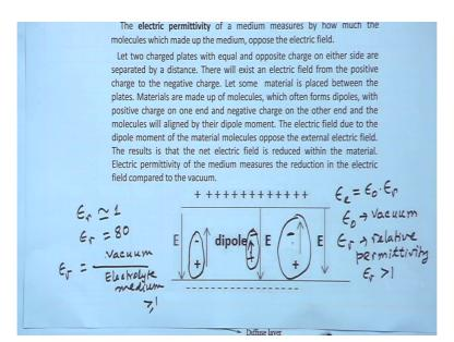
So when you have a medium over here, say suppose you have two charged plates positively charged and negatively charged and there is a medium and so there will be electric field will be generated this mediums is composed of some water or something. So that will from a dipole to oppose the medium is made up of molecules of course so they will form it, each molecule will form a dipole to oppose the electric field.
