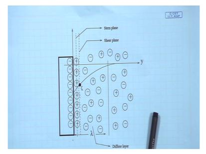
So, Now if I show in this figure, so this is the surface charge develops which is negative and it will attract positive ions from the aqueous media, so there will be a situation like this, so then this positive electron negative ions and in that process. There will be a layer near the surface where there will be a more number of unbalanced charged ions and compared to the bulk or core region.
