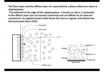
So if there is an external mechanism applied so okay, whatever was here so then what will happen? this positive ions will get attracted to the negative electrodes, say so if I apply say if I take a cathode anode here and there is a cathode here so that is called this is anode this is cathode. Now so this is the Devilier, so now if there is a voltage electric field is applied that is creating a voltage drop.
