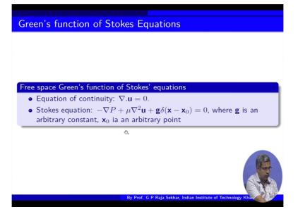
So we have the corresponding mass conservation and then stokes equation but not the homogeneous one. We are considering a point source on the right hand side with a strength g bar. Now we would like to compute the singular solution of this okay. So if you recall in the week 3 we discussed a singular solution of stokes equation but restricted to irrotational. That is due to potential flow.
