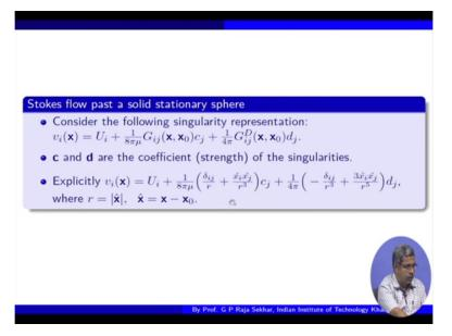
Which means we are considering the flow is far field is uniform, then a Stokeslet and a potential dipole okay. So it is slightly the tensor notation etc., slightly difficult but this is just to give you an idea. Now c and d are the strengths of the singularity. That means c bar is the strength of the Stokeslet, d bar is the strength of a dipole potential dipole okay. So how do we determine c bar and bar. Simply you force the no slip condition okay.
