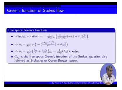
And in index notation we can write ui is this. The same expression the same u in index notation we can write okay. Then we simplify this we are operating the derivative on r and then next derivative we are operating on r. So we try to simplify and what we get is finally the free space Green's function of stokes equation okay. So this is a in a slightly complicated manner but this is a arbitrary solution.
