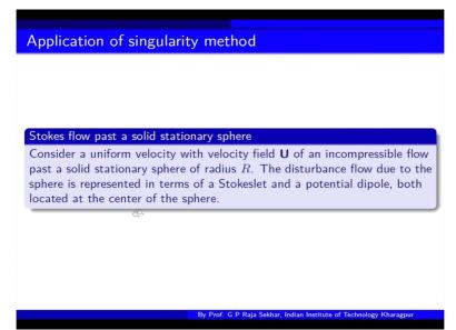
So let us consider that as an okay. So let us consider as an application of singularity method Stokes flow past a solid stationary sphere. So what we are considering? A uniform velocity okay U bar and then a sphere of radius R. Our aim is to compute the drag force which is the strokes drag. Now typically in the separable solution we have shown that we have considered corresponding stokes stream function and uniform flow added disturbance and computed to the separable solution right.
