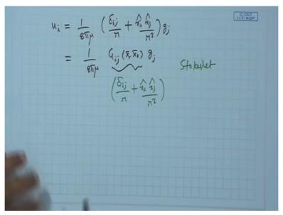
So what we are getting is. So this in tensor notation typically we write it. So where this denotes the tensor and this particular. So P already we have got okay, so this particular solution is called Stokeslet. Then similar to the potential case if you differentiate the corresponding the higher-order single solutions of Stokes flow can also be obtained okay.
