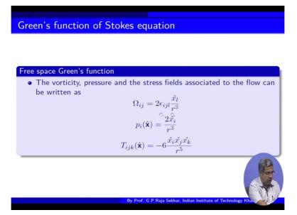
So corresponding to the Stokeslet that means if this is the velocity of Stokes flow, then the pressure is given by this stress field is given by this and the vorticity is given by this okay. Now I promised that I will show some application of a singularity method okay. So we will consider correspondingly will consider the corresponding Stokes flow past a sphere that we have done already.
